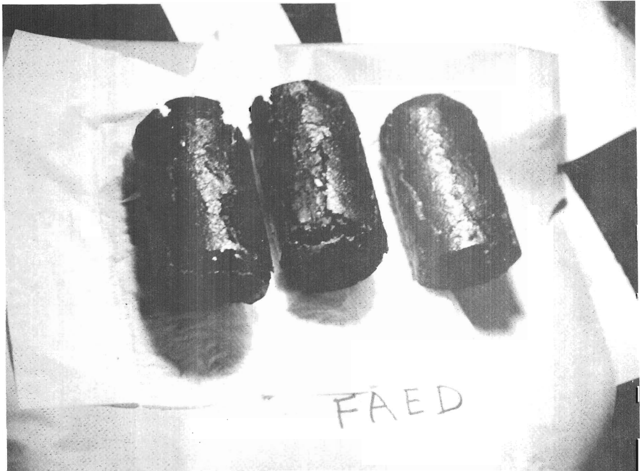
Figure 2.—Swelling and splitting of furfural acetone epoxy polymer concrete in 5-percent sulfuric acid. Photo P801-D-80332.
