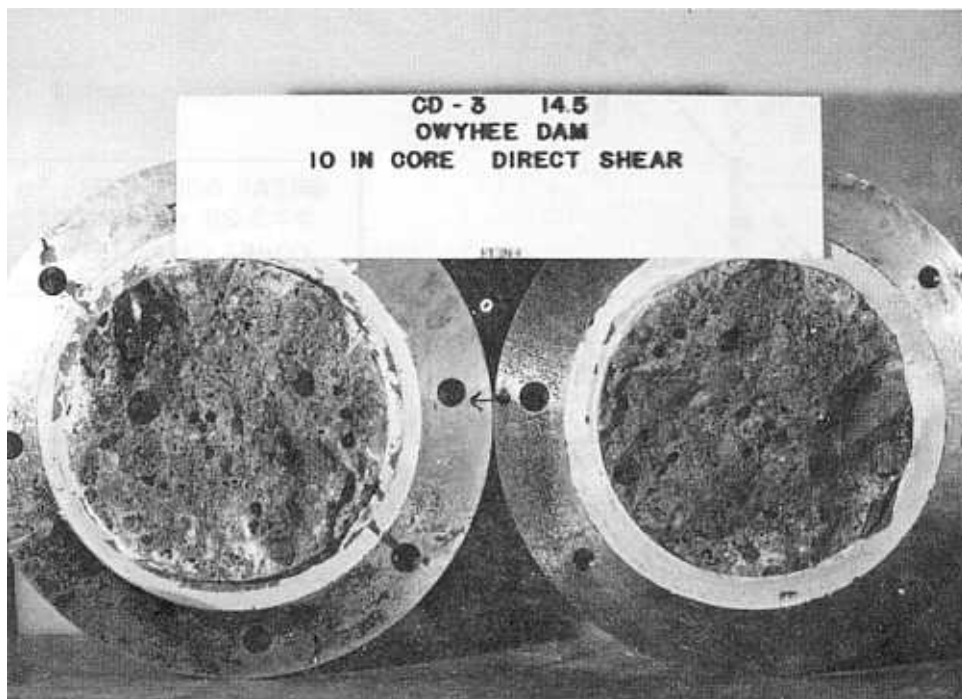
Figure 10. — Typical direct shear test specimen after test. Owyhee Dam. P801-D-80040
