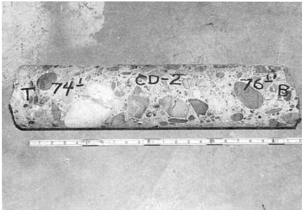
Figure 2. — Typical concrete core test specimen. Owyhee Dam. P801-D-80038
