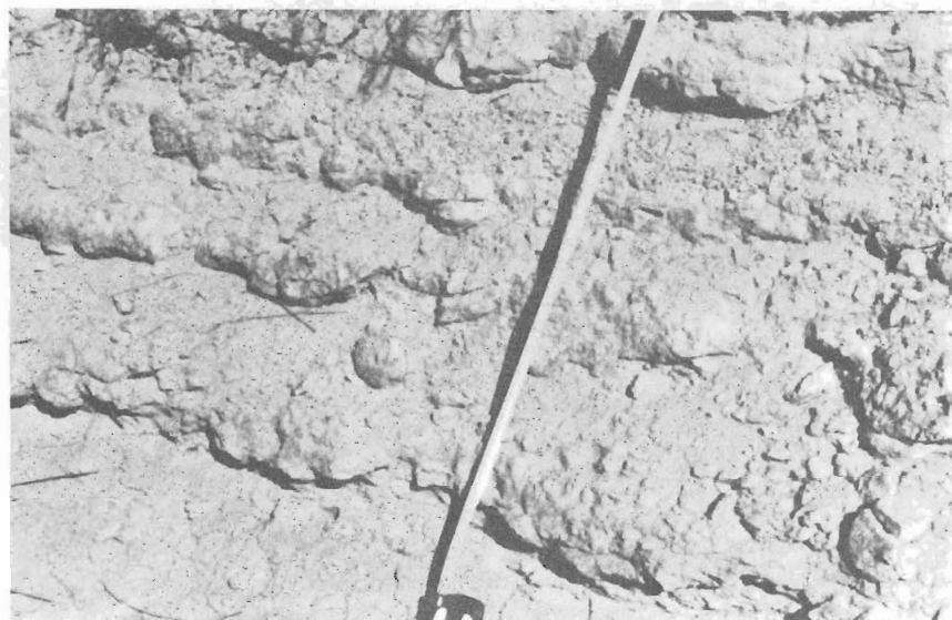
Figure 9. — View of 4.5 percent cement-modified soil near station 299+82. P801-D-80031.
