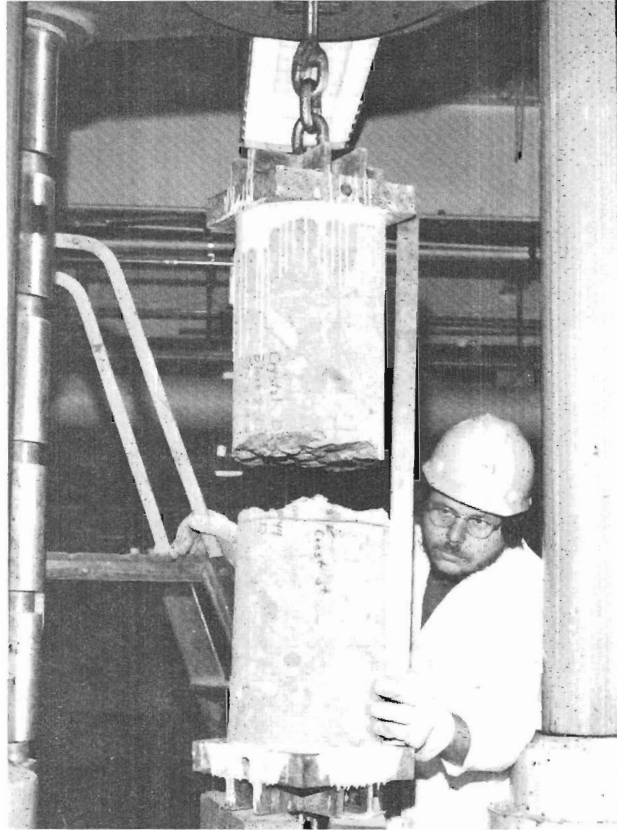
Figure 4. - Typical 250-mm (10-in) diameter core after tensile strength test - Crystal Dam. Photo C-8448-1.
