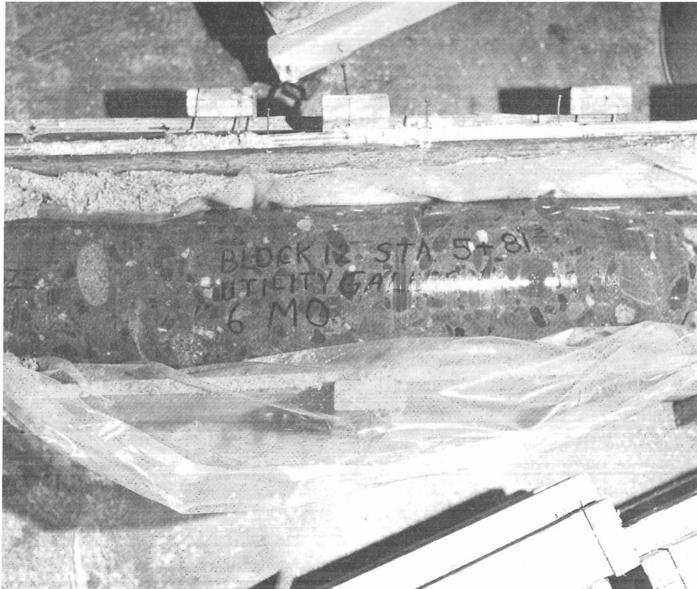
Figure 2. - Typical "as-received" condition of 250-mm (10-in) diameter cores - Crystal Dam. Photo Pb22C-427-7363.
