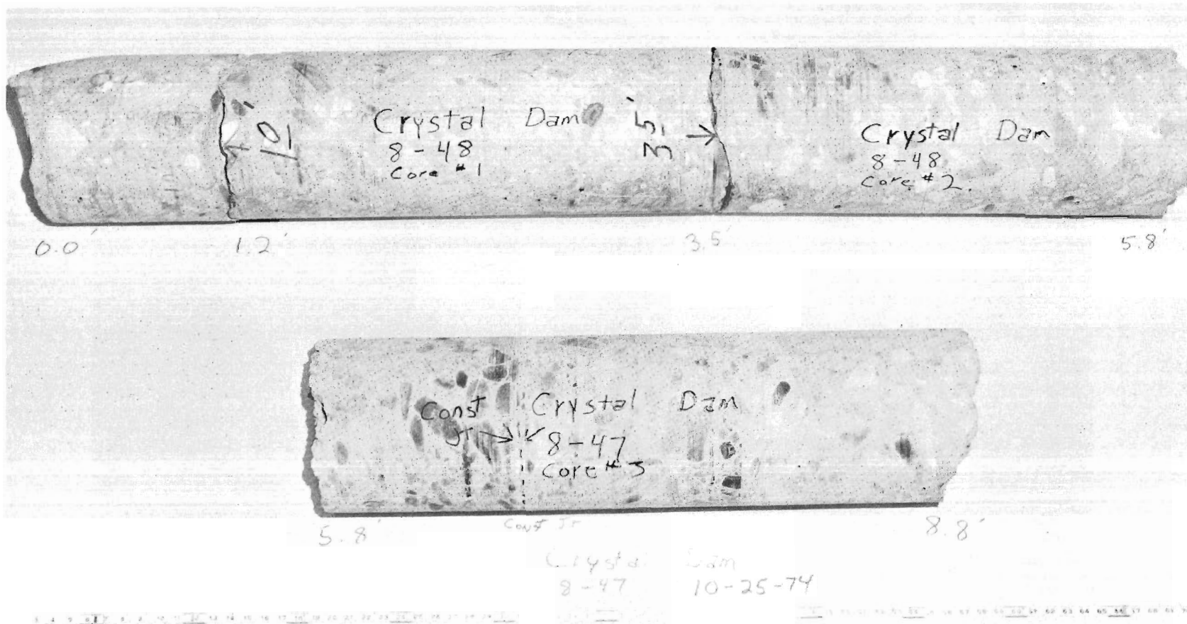
Figure 3. - Typical 250-mm (10-in) diameter cores showing a construction joint - Crystal Dam. Photo C-8426-2.
