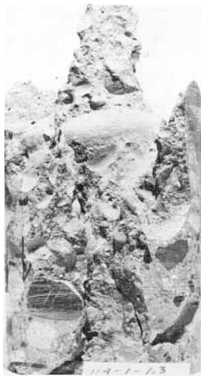
Figure 3 - Photograph of concrete showing failure surface Top - jointed concrete 1,000 psi lateral load (note jagged break) Bottom - unjointed concrete "0" lateral load (cone shaped break) C-8322-57 C-8322-56
