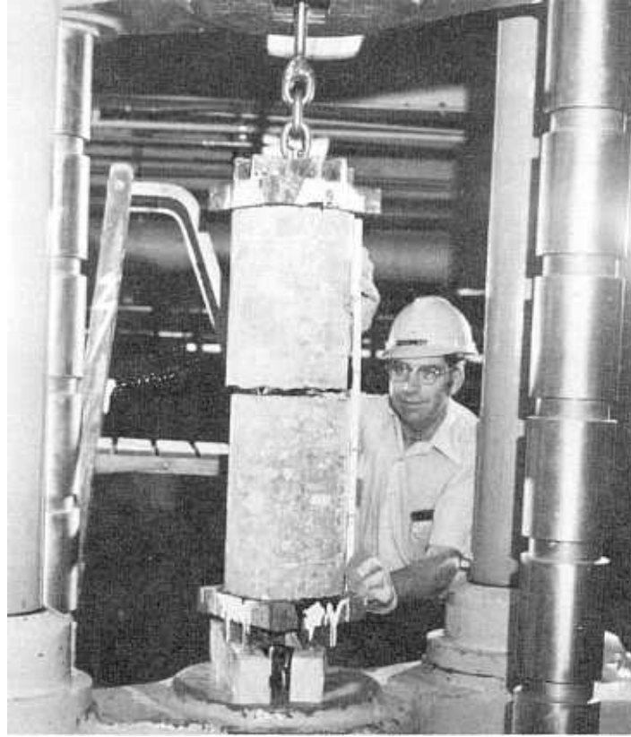
Figure 3. - Typical 255-mm (10-in) diameter core after tensile strength test - Grand Coulee Forebay Dam. Photo P1222-D-78273
