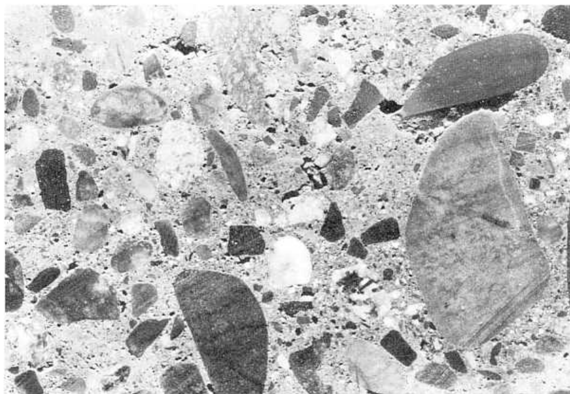
Figure 7. - Photograph of concrete showing size of aggregate and distribution indicating possible joint planes
