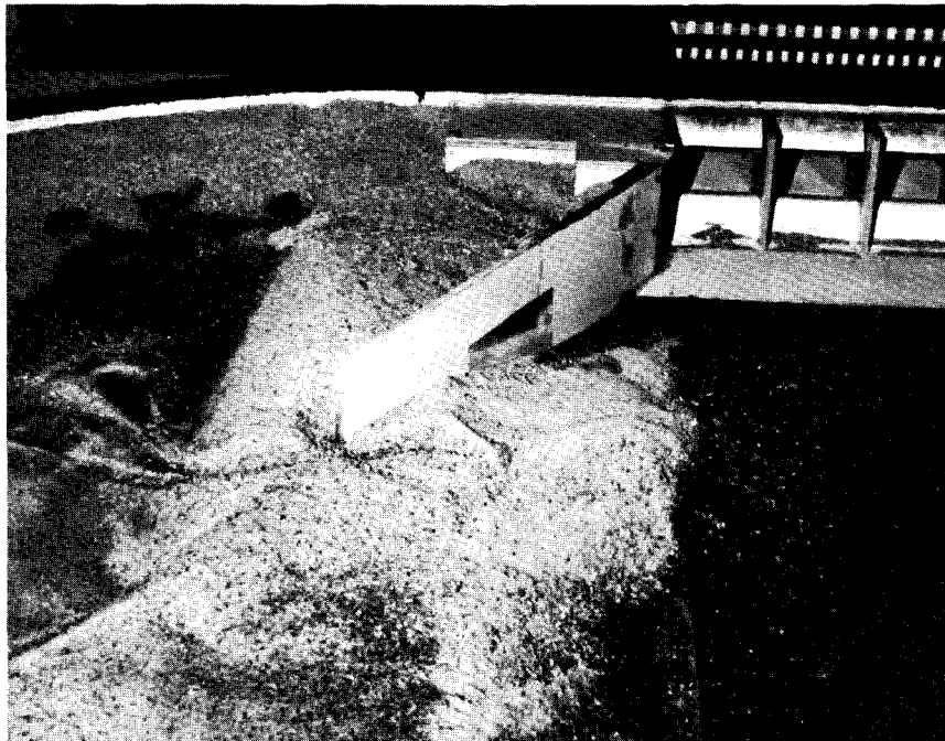
Figure 9.—Scour around left 30° wingwall with 100-m dike, Q_p = 7080 \text{ m}^3/\text{s} for 8.94 hours. P801-D-79821
