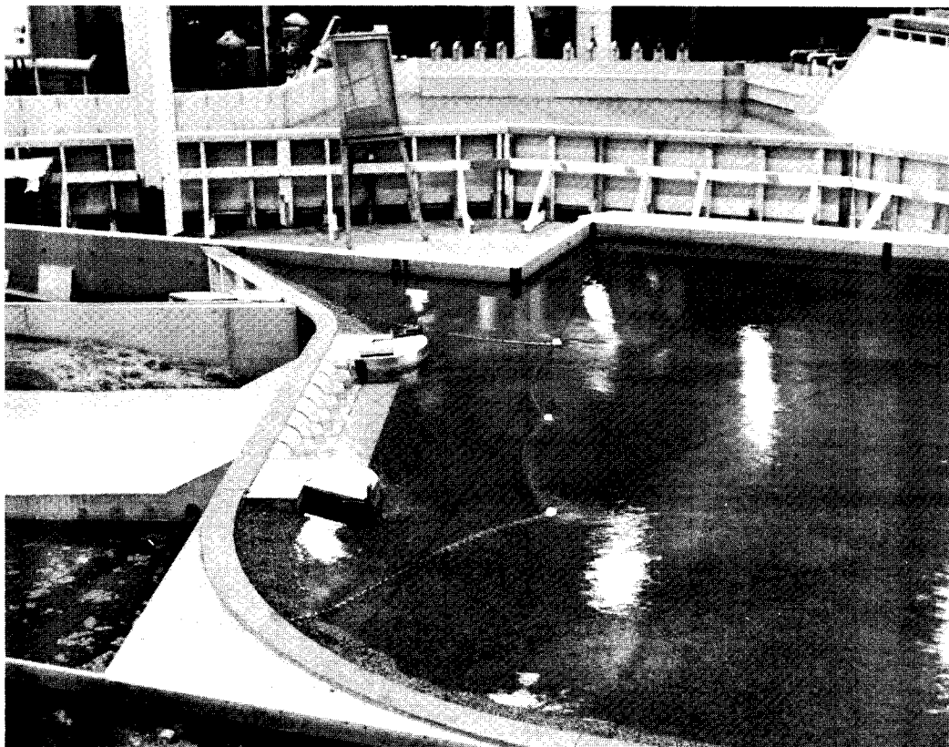
Figure 25.—Choke Canyon Dam model safety boom in place, Q_p = 7080 \text{ m}^3/\text{s} . P801-D-79836
