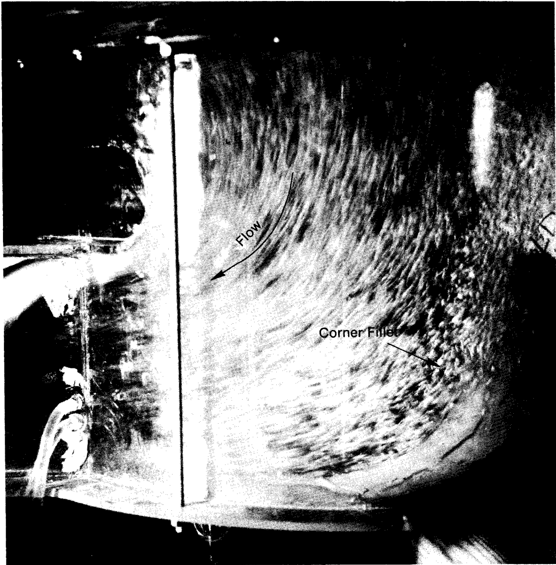
Figure 13.—A 2.43-m-radius fillet placed between upstream tower wall and tower floor (one fillet on each side of tower), reservoir EL = 1460.2, Q = 107.5 \text{ m}^3/\text{s} . Photo 80308
