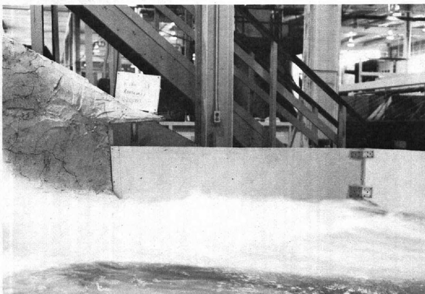
Figure 20.—Preferred design of lower training wall operating at 20 000 ft 3 /s (566 m 3 /s). P801-D-79569
