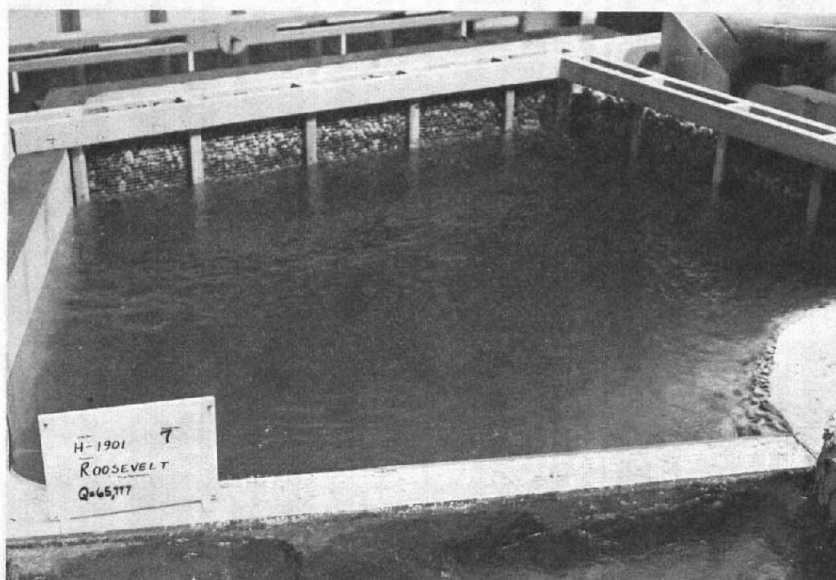
Figure 12.—View from spillway crest looking at dam access bridge. Q = 65\,777\text{ ft}^3/\text{s} ( 1862\text{ m}^3/\text{s} ) maximum discharge. P801-D-79564
