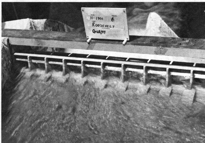
Figure 14. —View of model spillway gates in operation. Q = 65\,777\text{ ft}^3/\text{s} ( 1862\text{ m}^3/\text{s} ). Note severe contractions in bays 8, 9, and 10. P801-D-79565
