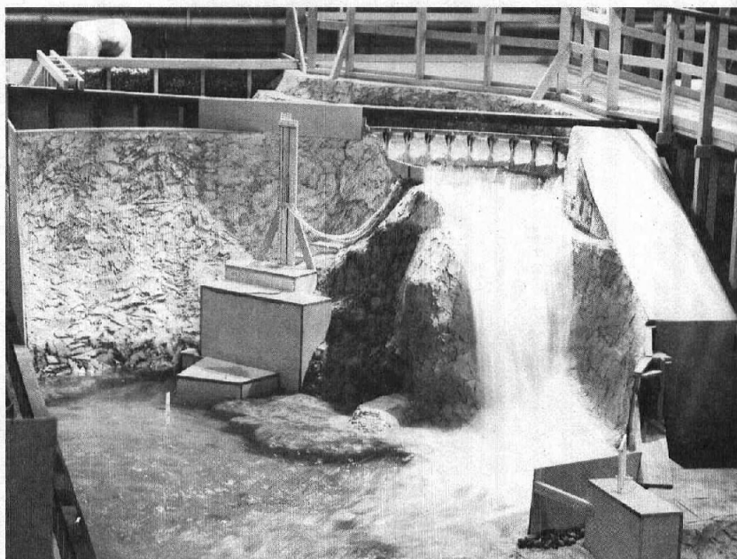
Figure 7.—Completed hydraulic model in operation. P801-D-79560
