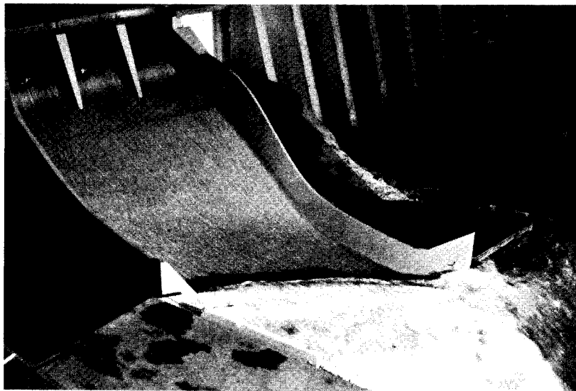
Figure 24. —Minimum spillway discharge flipping over lip, reservoir elevation 548.0 m (1798 ft), Q = 356.8 \text{ m}^3/\text{s} (12 600 \text{ft}^3/\text{s} ). Photo P801-D-79509
