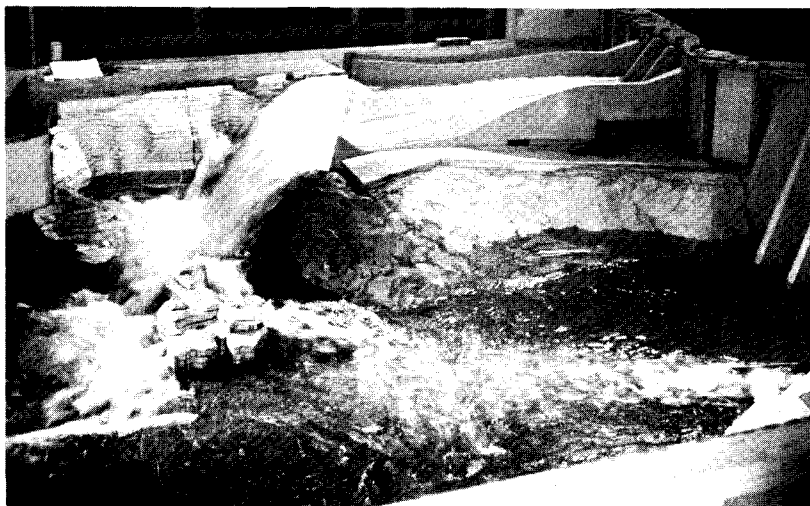
Figure 14.—View of spillway chute and plunge pool (test series "B"), 1982 m 3 /s (70 000 ft 3 /s). Photo P801-D-794501
