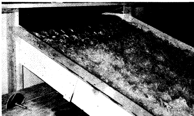
Figure 11.—Spillway flows for selected discharges with first row of blocks.
