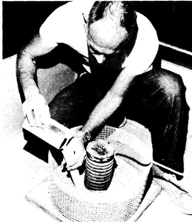
(a) Placing the gravel. Photo P801-D-79027
