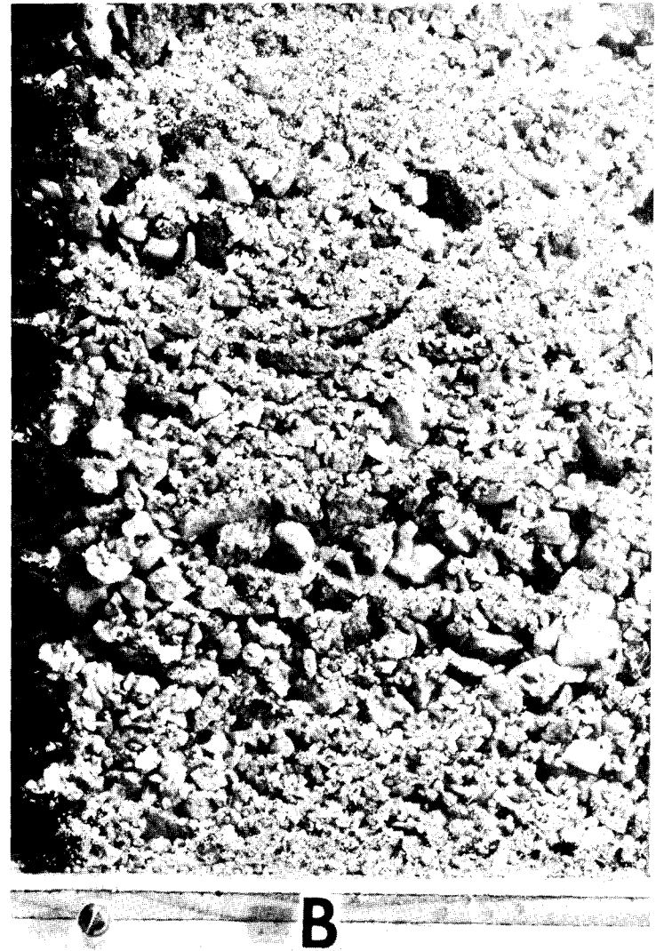
Figure 15.-Voids adjoining the corrugations. Photo P801-D-79031
