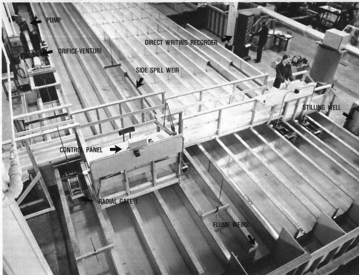
Figure 6.—Control panels, flume, and side spill weirs of canal model. Photo P801-D-77756
