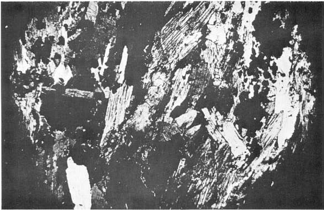
Plate 1. Photomicrograph of Muscovite-biotite Schist (P-7075) composed of coarse-grained euhedral mica (showing cleavage planes) and anhedral quartz. Minor sillimanite, clay and iron oxide also occur. The grains are poorly interlocked and the rock is well foliated. Polarized light Magnification 10X Photo PX-D-36283
