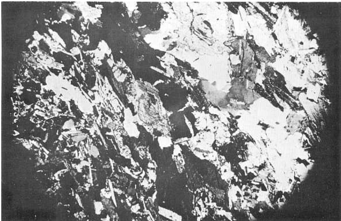
Plate 2. Photomicrograph of Mica-quartz Schist (P-7074) composed of medium-grained euhedral mica and anhedral quartz. The grains have smooth grain boundaries and are poorly interlocked. The mica is frequently aligned. Polarized light Magnification 10X Photo PX-D-36284
