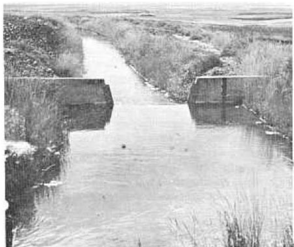
Figure 18. Cipoletti weir operating with good flow conditions in the approach pool. Flow is well distributed across wide pool and shows no evidence of excessive turbulence. Accurate or "standard" discharges can be expected under these conditions. Photo POAX-D-18350
