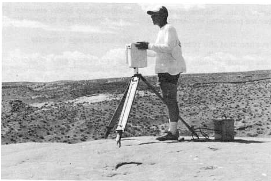
Figure 11. – Microwave receiver-transmitter at shore station. P801-D-81399
