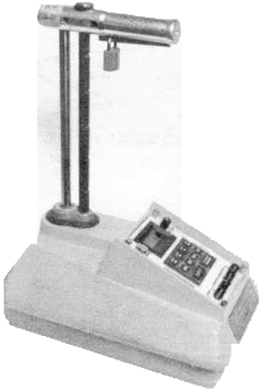
Figure 14. — Troxler 3411B nuclear gauge. Used for moisture and unit weight determinations. P-801-D-81155
