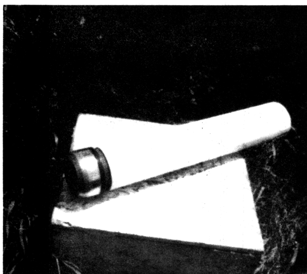
Figure 6. – Liner made from cut section of 5-inch (13-cm) i.d. PVC pipe. P-801-D-81149
