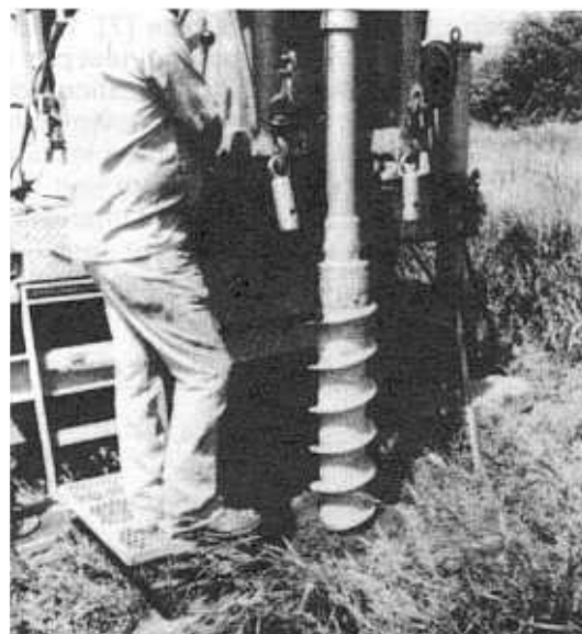
Figure 4. – Hollow-stem auger system. A 10½-inch (27-cm) o.d. flight auger with 6¼-inch (15.9-cm) i.d. hollow stem. P-801-D-81148
