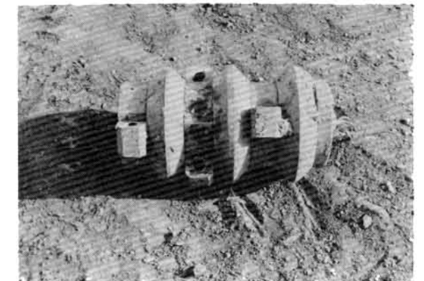
WORN TRI-DISC CENTER CUTTER
