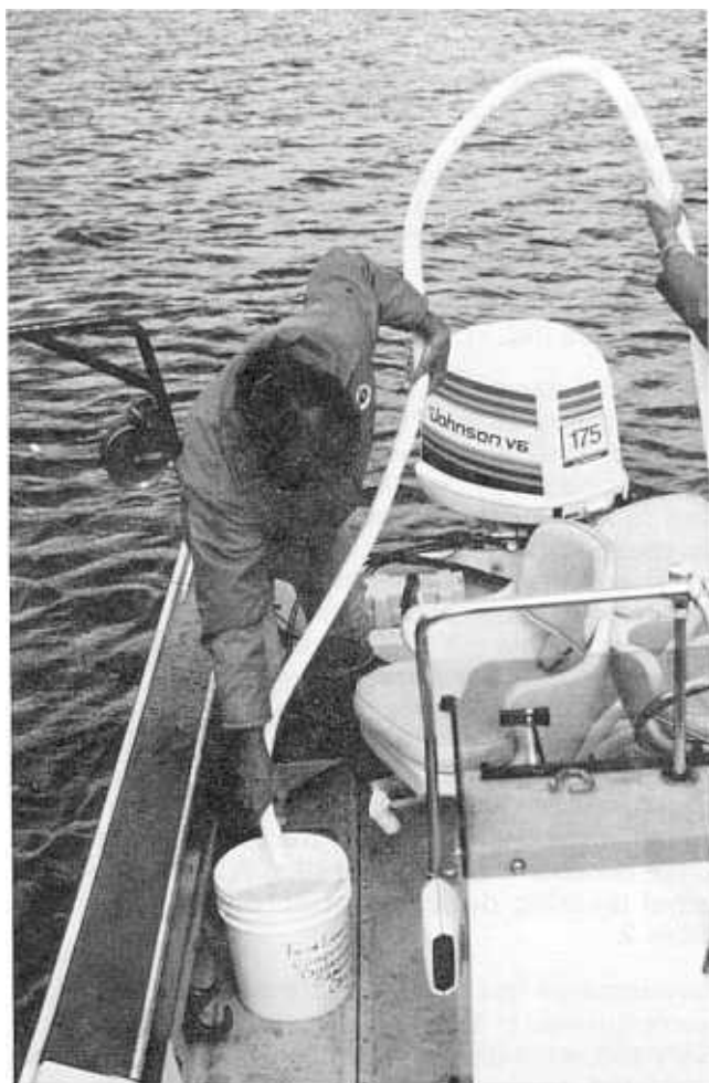
Figure 3. – Composite water sampler used to collect water for chlorophyll analysis at Twin Lakes. P801-D-80955
