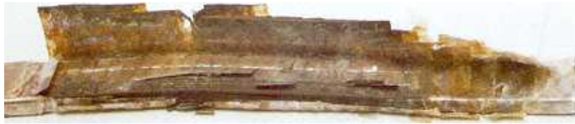
Figure 8.—Dissected coil prior to removal of all groundwall and turn insulation. P801-D-79795.
