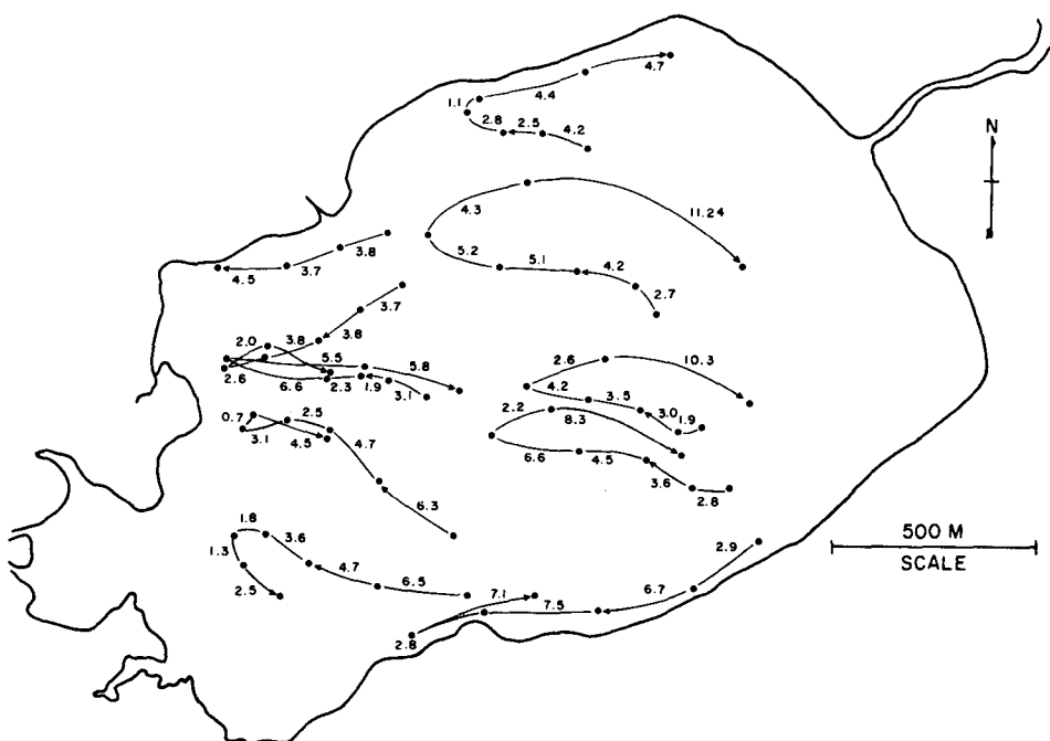
Figure 1-14—Surface currents measured on the upper lake, July 16, 1980. Velocities between drogue sitings are given in cm/s.
