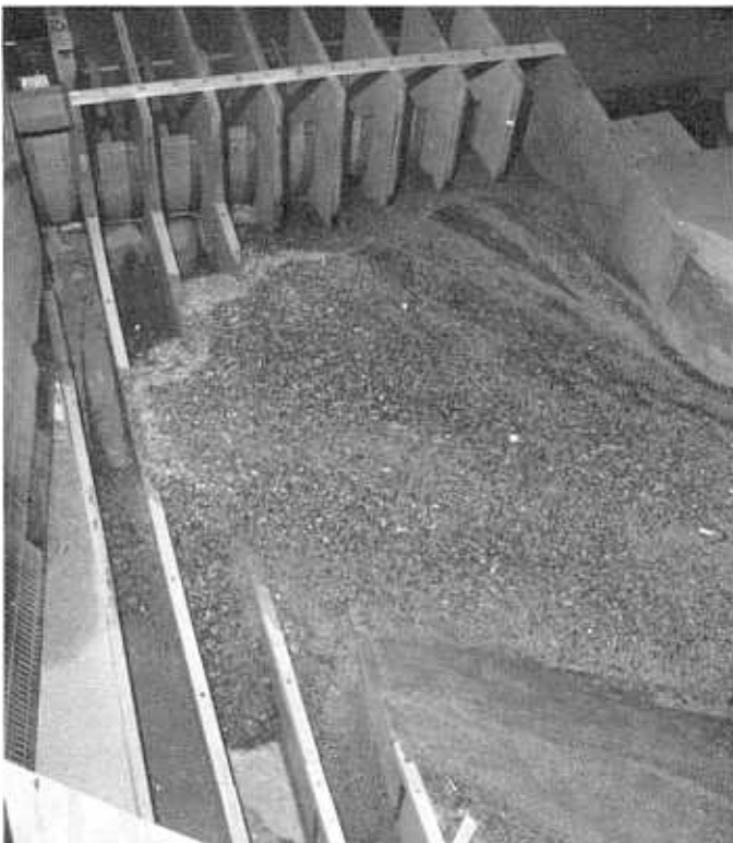
Figure 32.—Some sluicing-trap and spur-wall arrangements tested.
