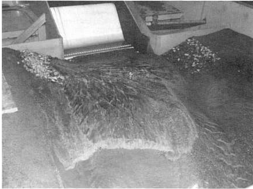
Figure 19.-The delta-front sediment bar traveling through the downstream river and weir approach channels. P801-D-79627
