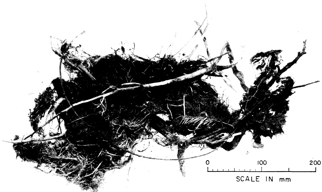
Figure 7.—Fine, submerged debris raked from trashrack. P801-D-79617
