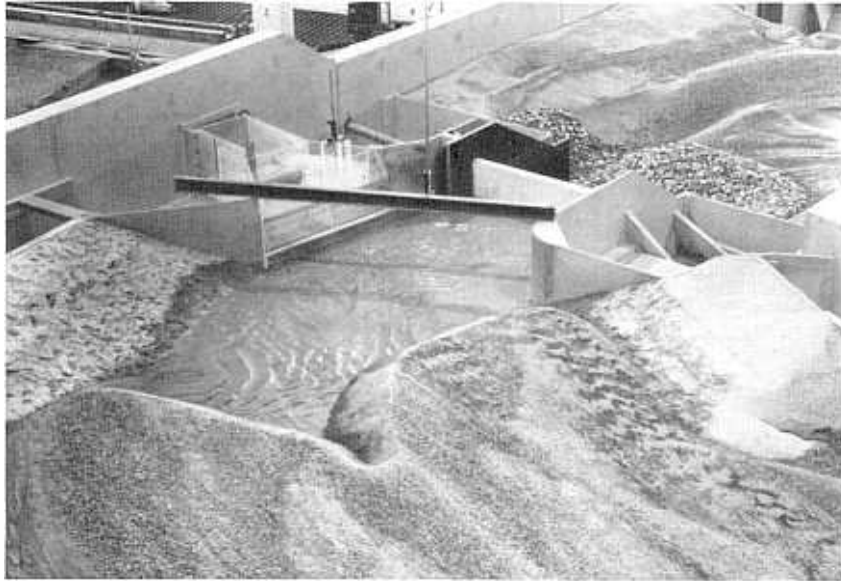
Figure 17.—The delta-front sediment bar approaching the diversion structures. P801-D-79625
