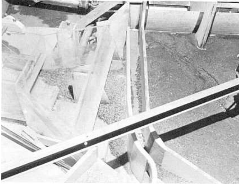
Figure 28.—Sediment that traveled into the original headworks during operation with the first modification. P801-D-79636
