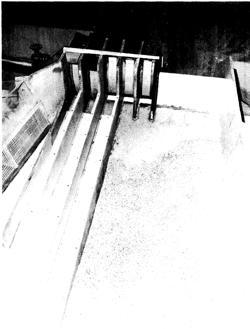
Figure 34.—Sediment traps of the recommended modification. P801-D-79640
