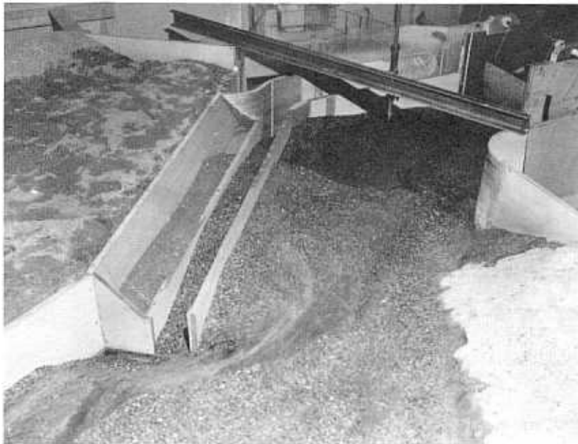
Figure 27.—Tunnel headworks and sluiceway of first modification. P801-D-79635
