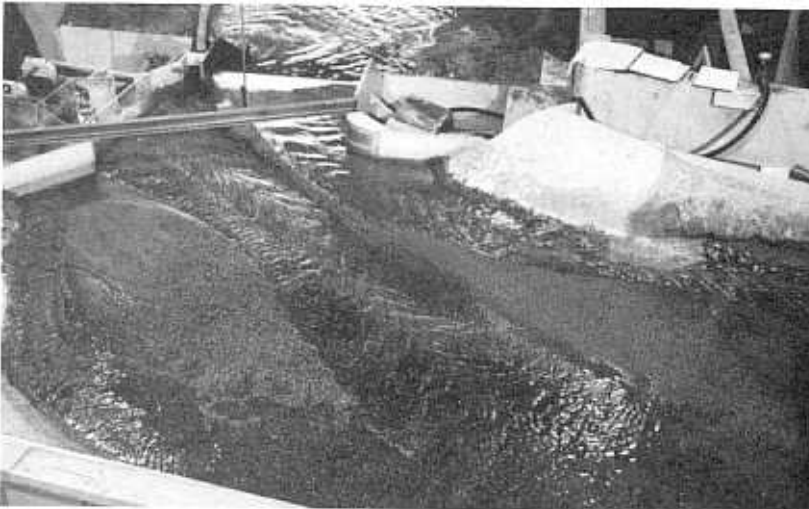
Figure 23.—Time sequence photographs before, various times during, and after cut-bank sluicing. (continued on next page)
