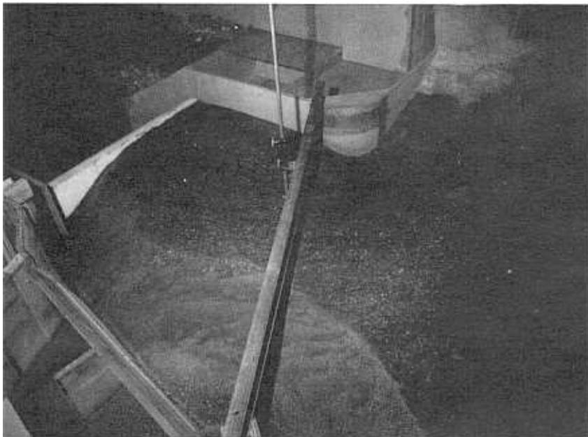
Figure 18.—The delta-front sediment bar after reaching the spillway. P801-D-79626
