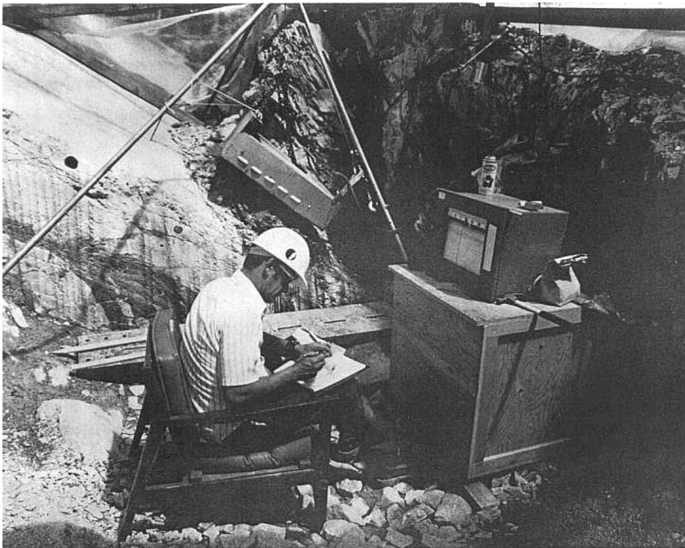
Figure 15. — Gas-fired, infrared radiant heater mounted over test site, and recorder monitoring temperatures. Temperature was sensed by eight thermocouples buried within the gouge. Photo P801-D-79262
