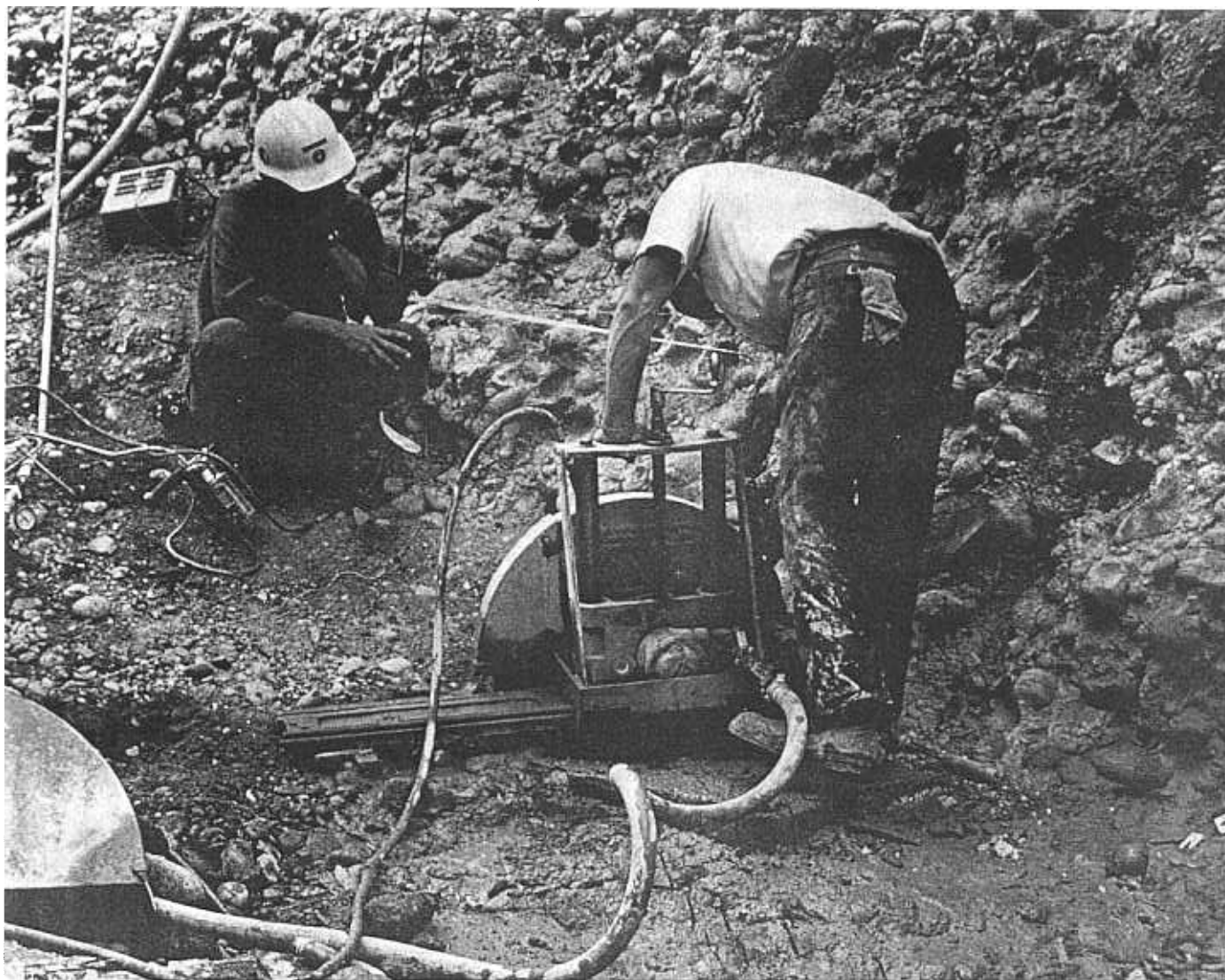
Figure 8. — A diamond-tip blade saw was used to make vertical cuts into the sample site. These cuts divided the site into slabs for removal and further study. Close observation also reveals several transverse cuts. Photo P801-D-79255
