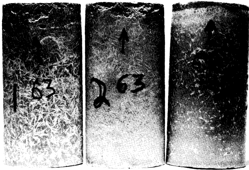
Figure 11.-Cylinders, 50 by 100 mm (2 by 4 in), cast for triaxial shear testing. W:C = 0.8:1, 6 percent calcium chloride, 27 to 32 °C (80 to 90 °F). Portions of outer layer, or crust, have separated from cylinders 1 and 2 (above arrows). Note white crystals. Small voids on cylinder 2 caused by crystals adhering to plastic mold. Photograph C-8481-142.
