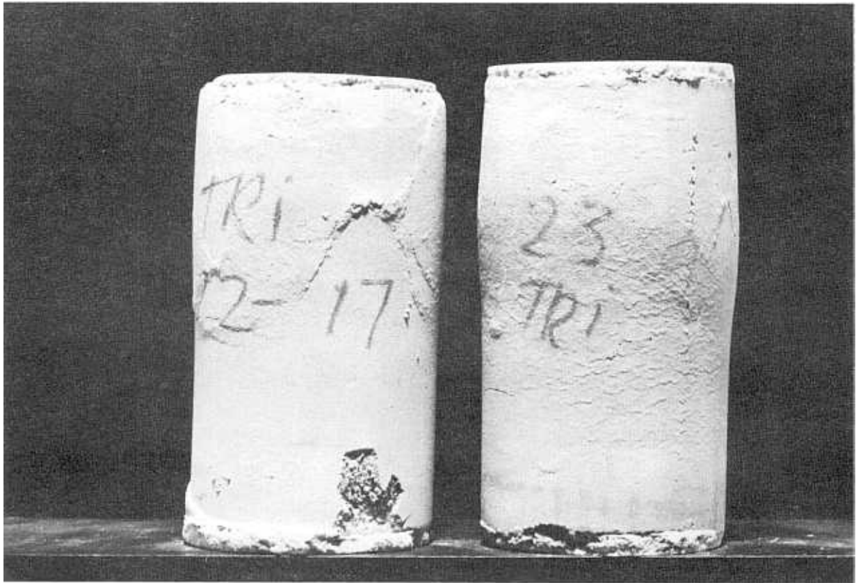
Figure 27.-Cylinders, 50 by 100 mm (2 by 4 in), tested for triaxial shear strength at an age of 90 days. Left: W:C:S = 1:1:1, 0 percent calcium chloride, 13 to 21 °C (55 to 70 °F). Right: W:C:S = 1:1:1.4, 0 percent calcium chloride, 13 to 21 °C (55 to 70 °F). Note bulging (i.e., strain) in horizontal direction. Planes of shear failure are evident. Photograph C-8481-148.
