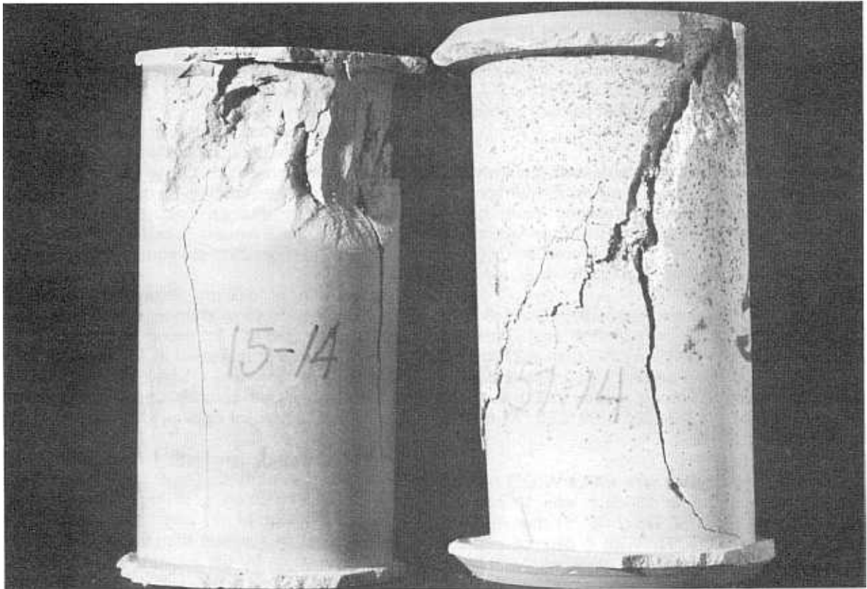
Figure 25.-Cylinders 50 by 100 mm (2 by 4 in), tested for unconfined compressive strength at an age of 90 days. Left: W:C = 0.8:1, 8 percent calcium chloride, 2 to 4 °C (35 to 40 °F). Right: W:C:S = 1:1:1.4, 6 percent calcium chloride, 2 to 4 °C (35 to 40 °F). Left cylinder shows splitting failure. Right cylinder shows shear failure on diagonal plane (roughly 1 o'clock to 7 o'clock). Photograph C-8481-116.
