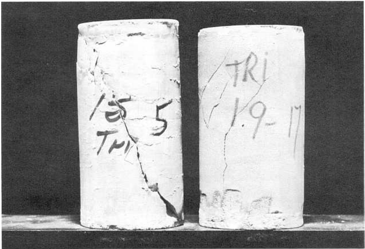
Figure 26.-Cylinders, 50 by 100 mm (2 by 4 in), tested for triaxial shear strength at an age of 90 days. Left: W:C = 0.8:1, 8 percent calcium chloride, 2 to 4 °C (35 to 40 °F). Right: W:C = 0.8:1, 0 percent calcium chloride, 13 to 21 °C (55 to 70 °F). Photograph C-8481-146.
