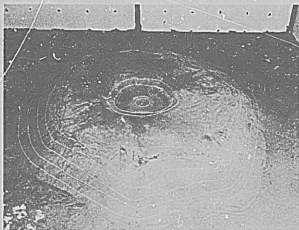
Figure 9. Test 7. Contours simulate 1-foot intervals, 0-6 feet, in prototype mine cavity after injection at 14.5 feet per second with slurry concentration of 16 percent. Photo P801-D-73846
