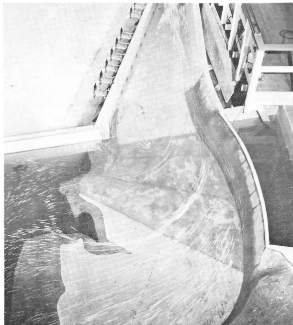
Figure 4. Flow pattern in preliminary forebay channel. Photo P1222-D-72992
