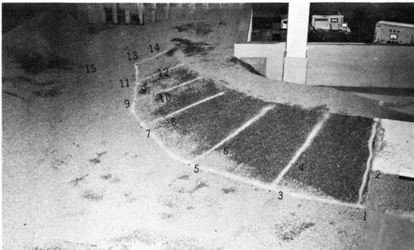
Figure 19. Velocity measurements in recommended 6-unit tailrace. Photo P1222-D-73007
