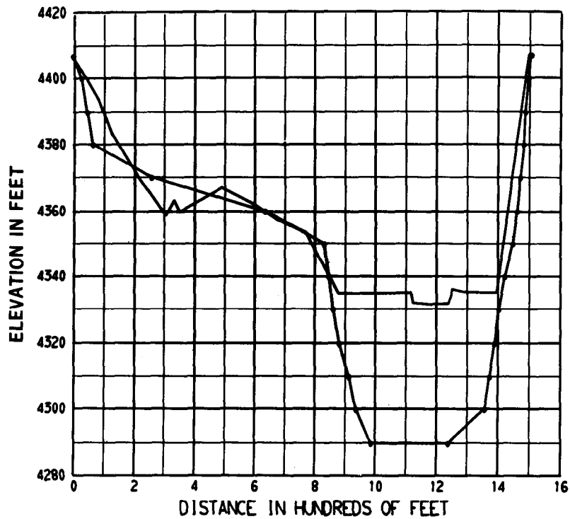
Figure 50. 1915 and 1969 sedimentation range profiles—Range 58.
