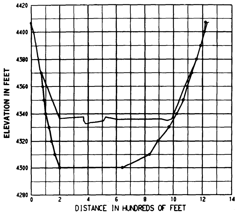
Figure 51. 1915 and 1969 sedimentation range profiles—Range 57.
