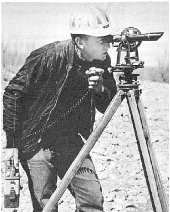
Figure 7. Man on shore keeps boat on line through radio communication with boat operator. Photo P24-500-1247 NA
