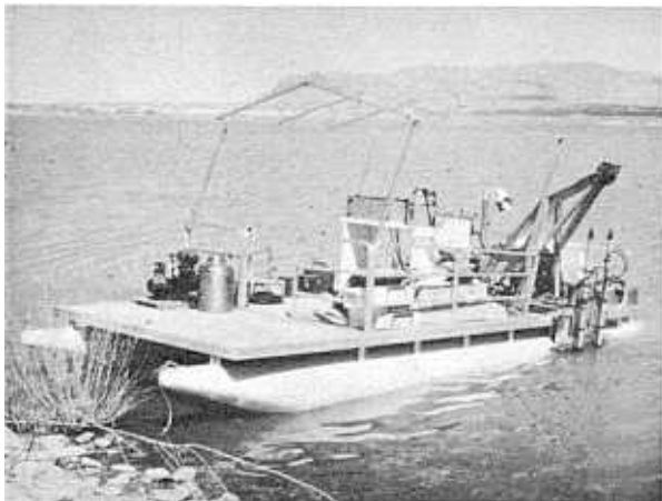
Figure 5. Equipment installed on deck of pontoon boat to run hydrographic survey.
