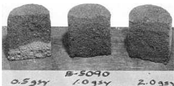
Photograph 2. Penetration of solvent-base stabilizers into 2- by 2-inch (5.1- by 5.1-cm) test cylinders at various application rates.
