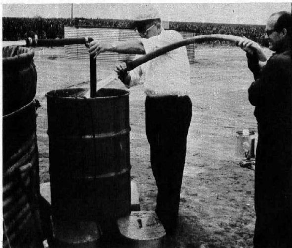
Photograph 5. Installation of soil sealants by ponding treatment method. The dry powder or slurry mixture, depending upon the sealant, was slowly added to the 55-gallon (208-liter) drum where it was continuously mixed and then pumped into the test tank. Photo P800-D-68965
