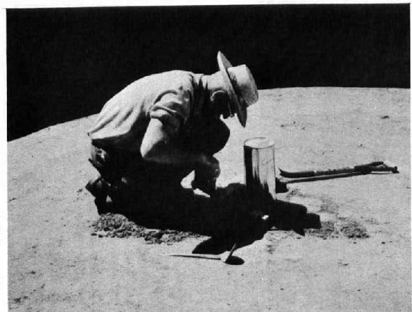
Photograph 3. Field density test using sand-cone method. Top photo P800-D-68961. Bottom photo P800-D-68962
