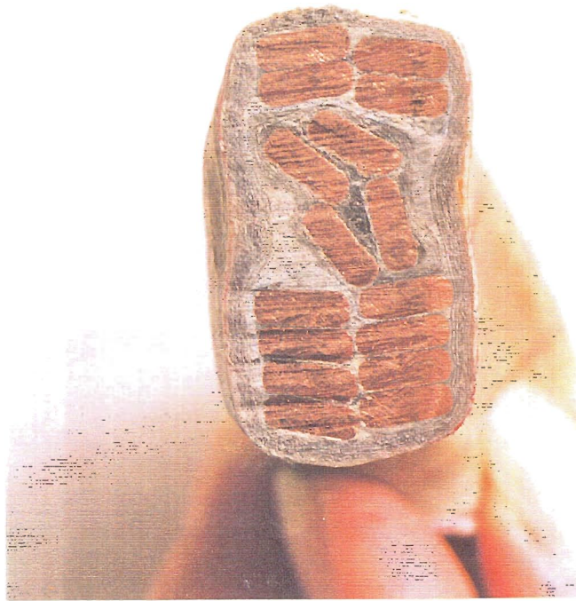
Photograph B.1. - Turn transposition.
