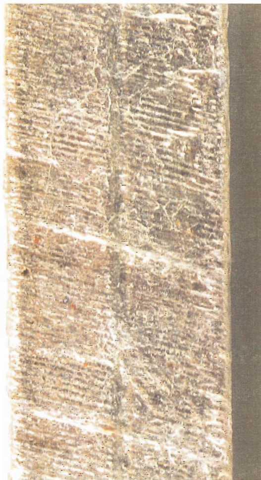
Photograph C.2. - Reddish-brown impurities in groundwall insulation.
