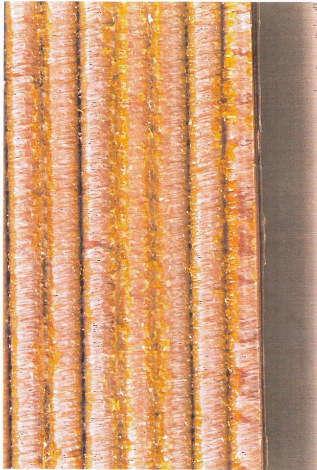
Photograph E.2. - Side view of conductor tier; shows voids in strand insulation and between adjacent turns.
