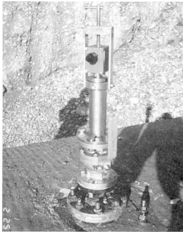
Figure 8. - Wet-tap hydrophone installation.
