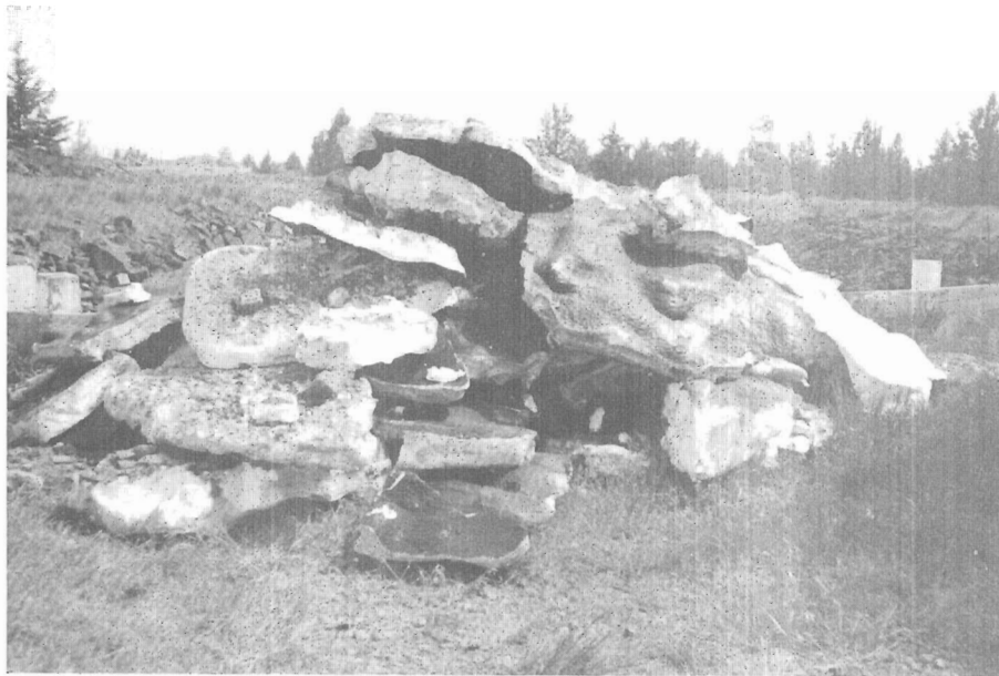
Photograph 54. - Several cubic yards of washed-out foam were collected at the siphon inlet.
