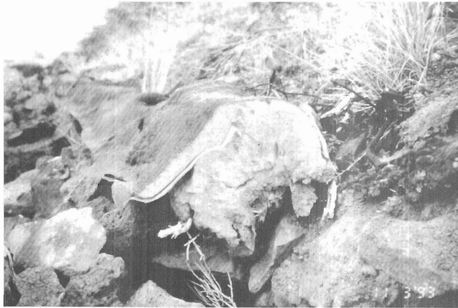
Photograph 63. - Geotextile liner tore parallel to foam anchor trench.
