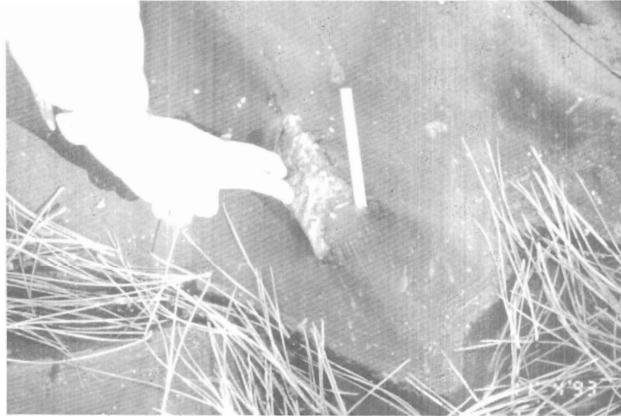
Photograph 37. - Tear over large sharp subgrade rock.
