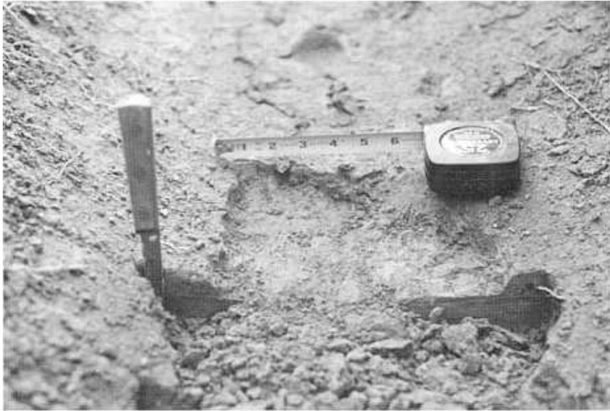
Figure 8. - Cross section of soil foundation of pipe No. 25 showing 1-inch-thick soil mound.
