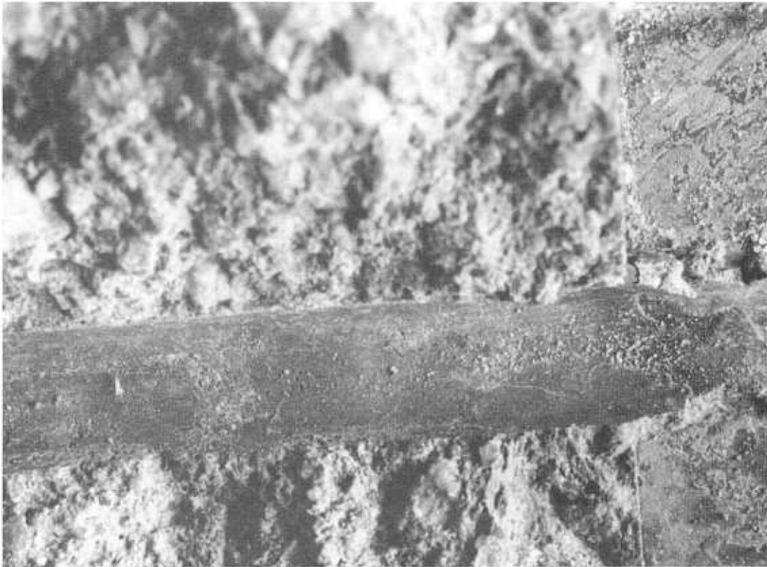
Figure 31. - Mortar coating opposite bell anchor, unit 798. Mirror image of wire fracture is imprinted, about 5.5X.
