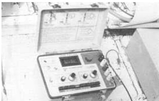
Figure 40. - A strain indicator was set and the initial strain reading was zeroed.
