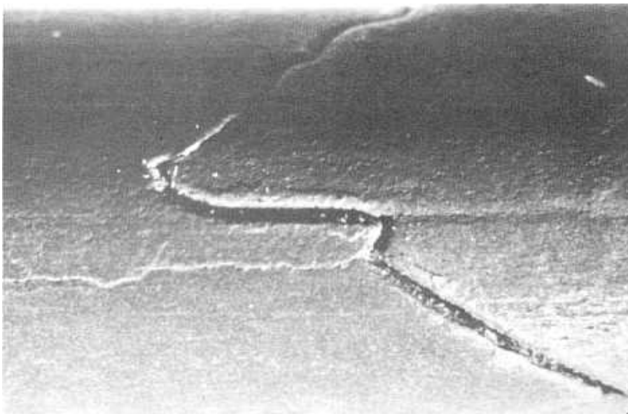
Figure 31. - Mortar coating opposite bell anchor, unit 798. Mirror image of wire fracture is imprinted, about 5.5X.
