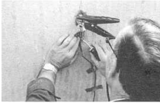
Figure 38. - A strain gage was spot welded to the prestressing wire in one hole while the wire remained stressed around the pipe under in situ tension.
