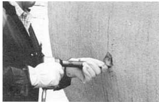
Figure 36. - Two holes were chipped in the mortar coating adjacent to each other in a line along the circumference of the pipe.
