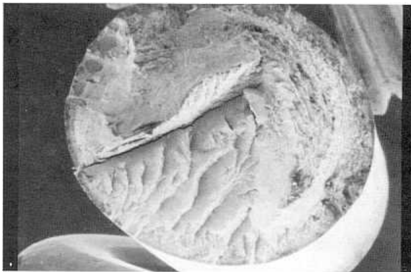
Figure 54. - Photomicrograph of surface in figure 53. Note the ledge or step transverse to the wire axis.
