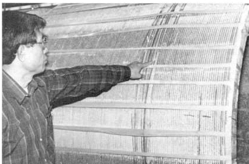
Figure 27. - Fewer and randomly located fractures were found on unit 798. The bonding straps were at the 5 and 11 o'clock positions on this unit in service.
