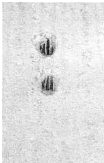
Figure 37. - The holes were separated by 1 inch of intact mortar coating and a minimum amount of prestressing wire was exposed for strain gage application.
