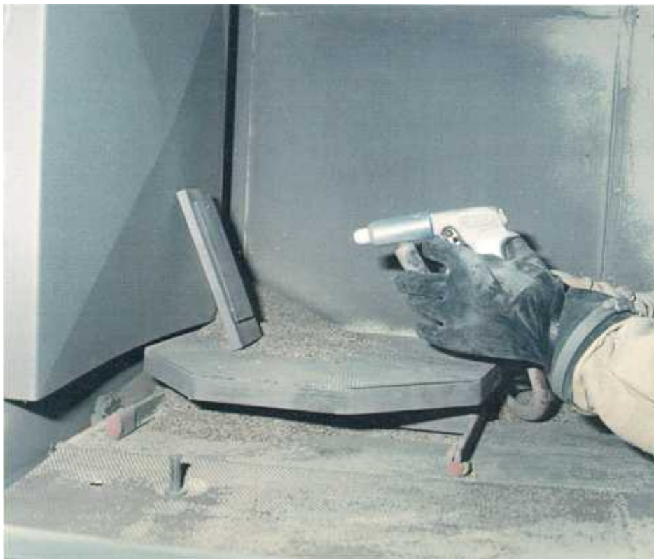
Inside view of the media blasting cabinet - panel preparation.
