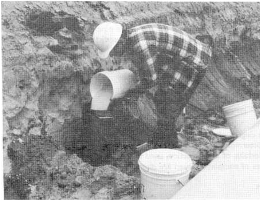
Figure 18. - Measuring in-place density using a sand cone device.
