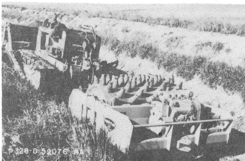
Figure B-10. - Vibratory roller used to compact soil in place.
