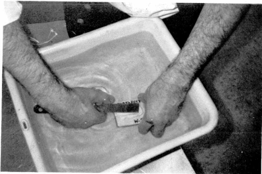
Figure 6. - Extensive tooling of the underwater specimens was needed to remove trapped water pockets, and promote good bond.
