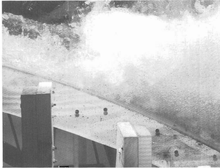
Figure 13. – As-built outlet works operating at 16.7-percent gate opening.
