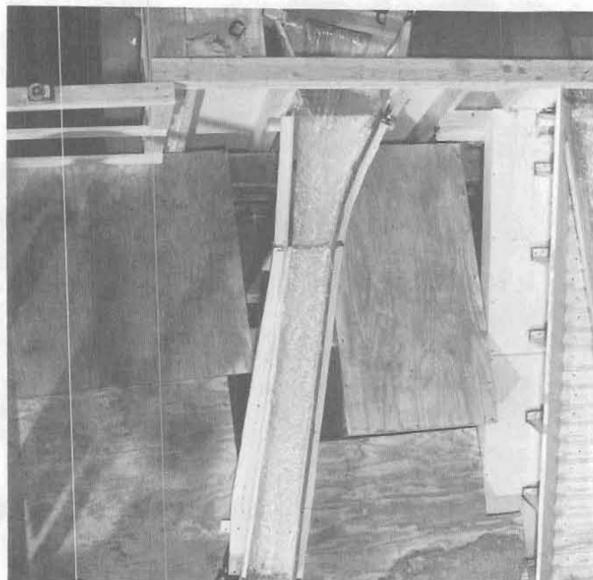
Figure 8. - Overtopping the left wall downstream of the crest (30- by 3.5-foot orifice).
