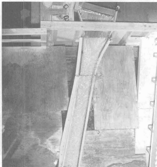
Figure 6. - Overtopping the left chute wall downstream of the crest for a discharge of 3,440 ft 3 /s through the 47.67- by 3.5-foot opening.
