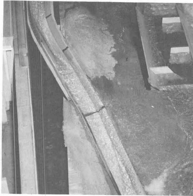
Figure 7. - Overtopping the left wall downstream of the horizontal bend for a discharge of 3,440 \text{ ft}^3/\text{s} through the 46.67- by 3.5-foot orifice.
