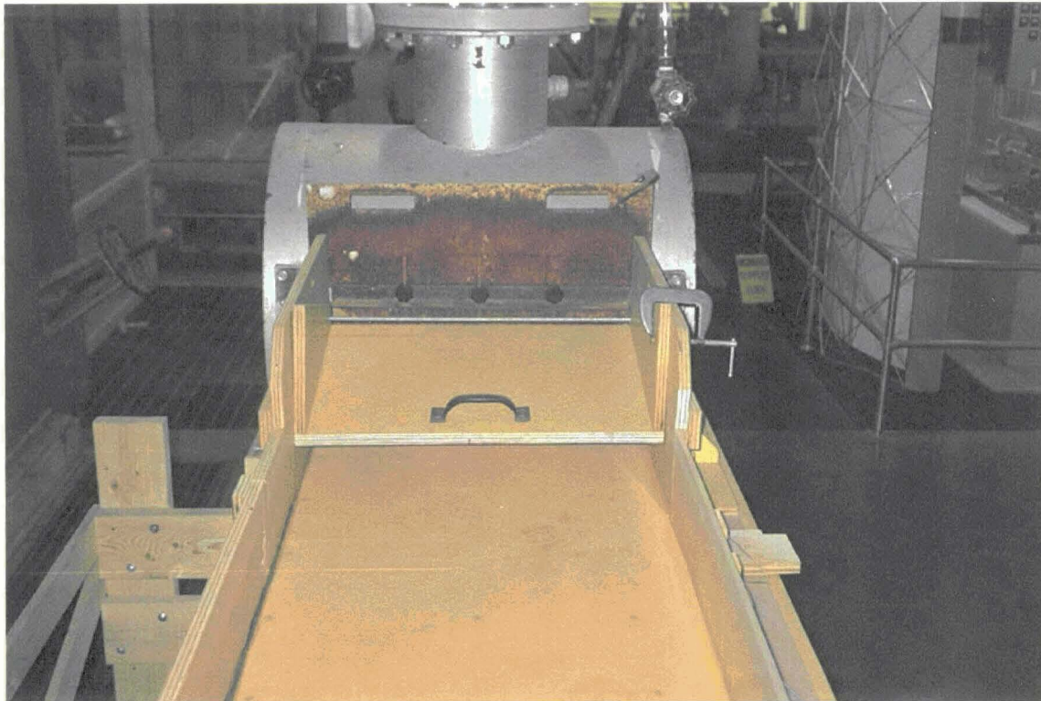
Figure 10.—Model head tank with slide gate and wave suppressor.
