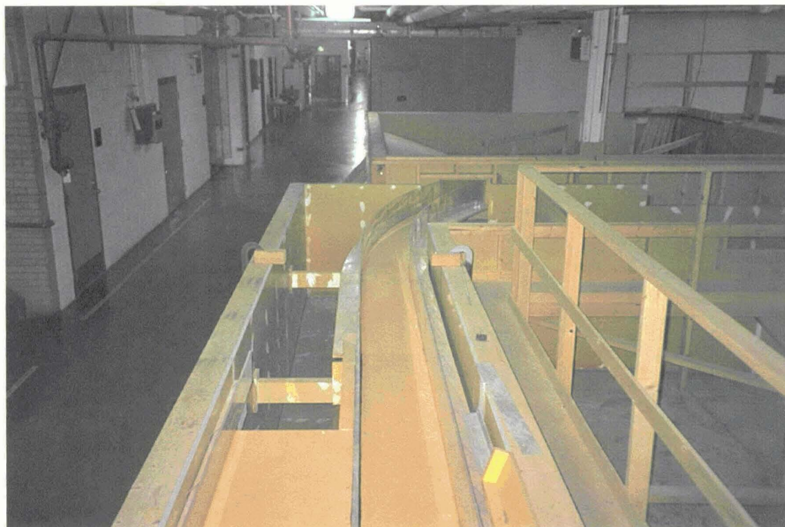
Figure 11.—Free overfall termination of model San Sevaïne channel with collector channel curving into model Jurupa Basin on the right.
