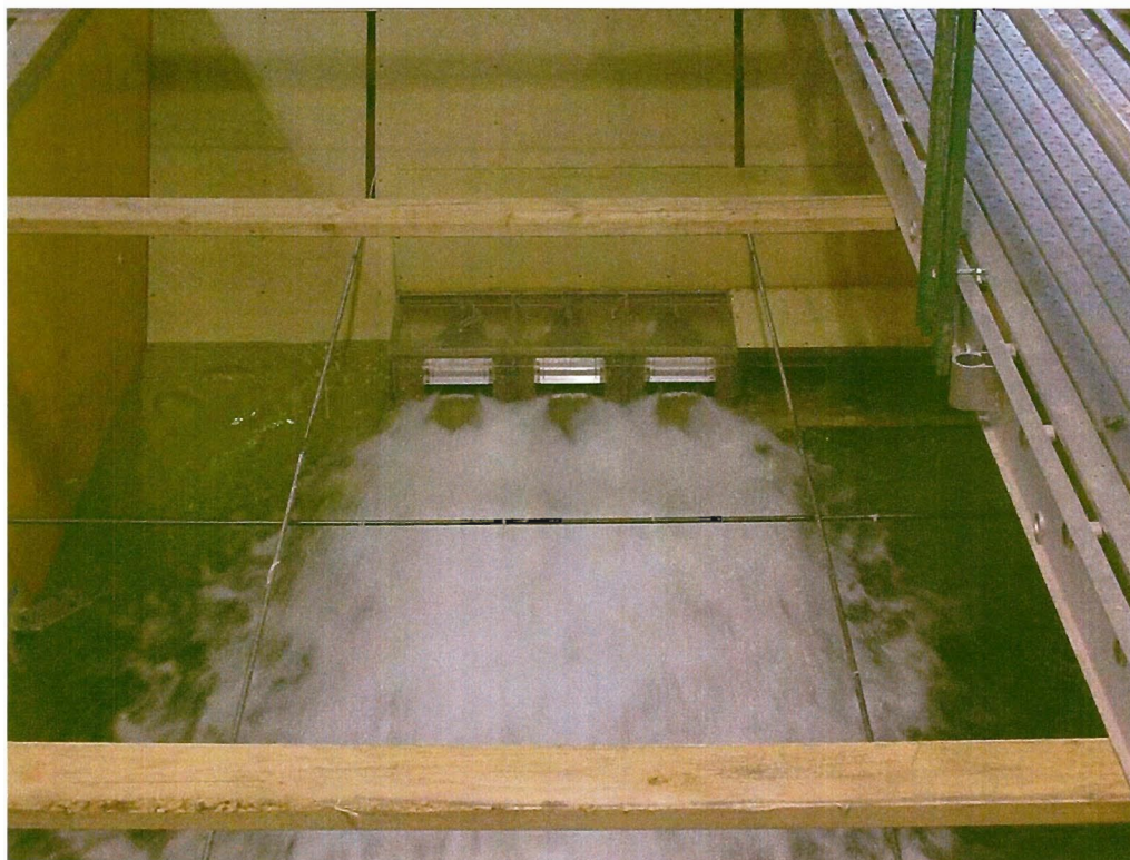
Three gates operated at 50-percent open under partial submergence.
