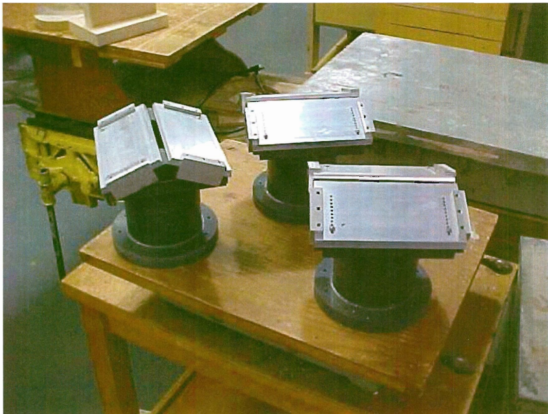
Figure 7. – Slide gate arrangement used to model the 48-in clamshell gates at 1:10.67 scale.
