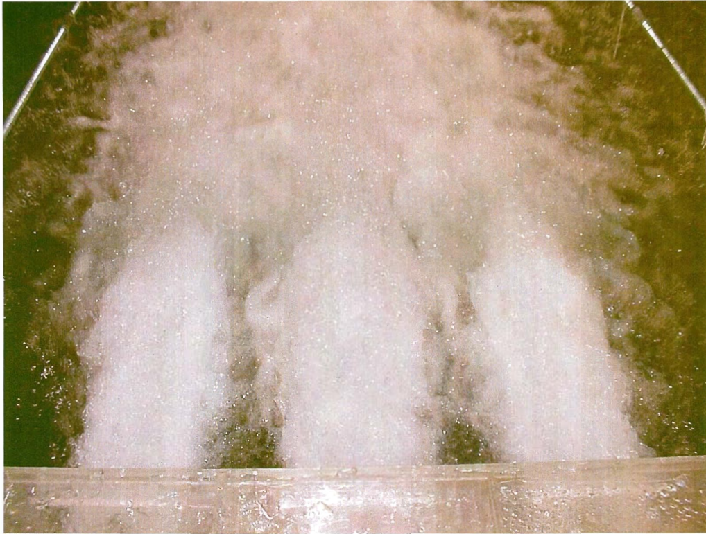
Three gates operated at 10-percent open under partial submergence.
