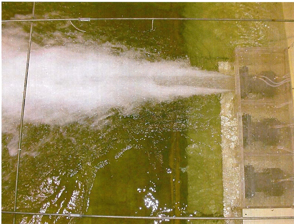
Single gate operated at 100-percent open under partial submergence.
