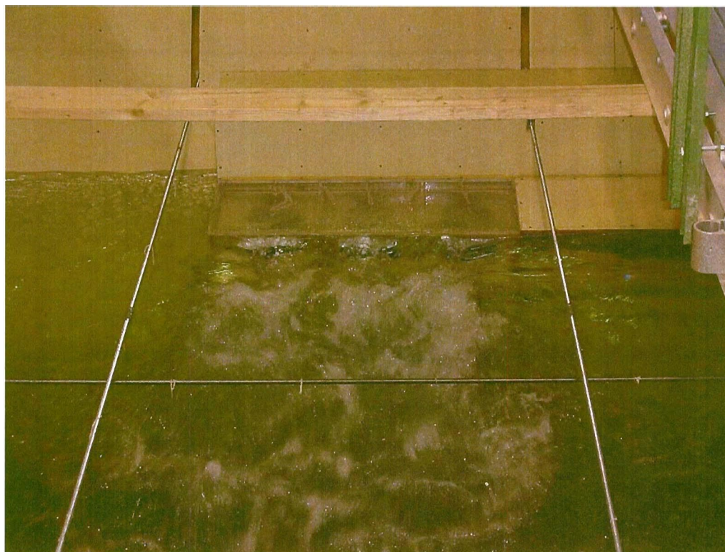
Three gates operated at 50-percent open under full submergence.
