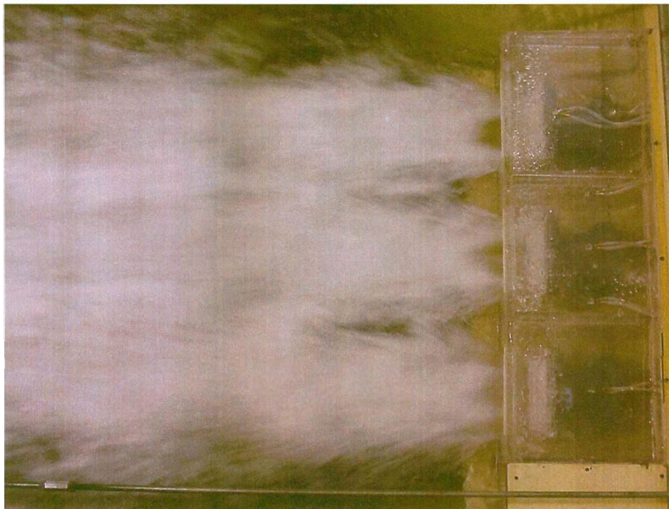
Three gates operated at 10-percent open under partial submergence.
