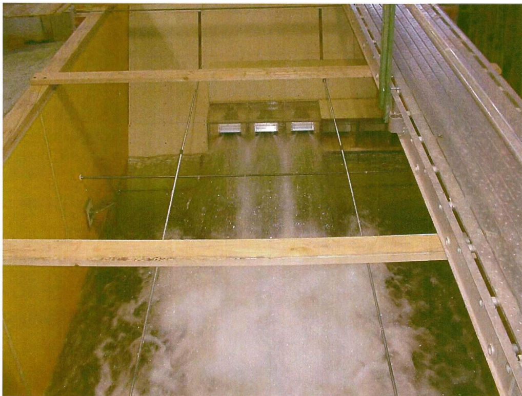
Three gates operated at 50-percent open in free-discharge mode.
