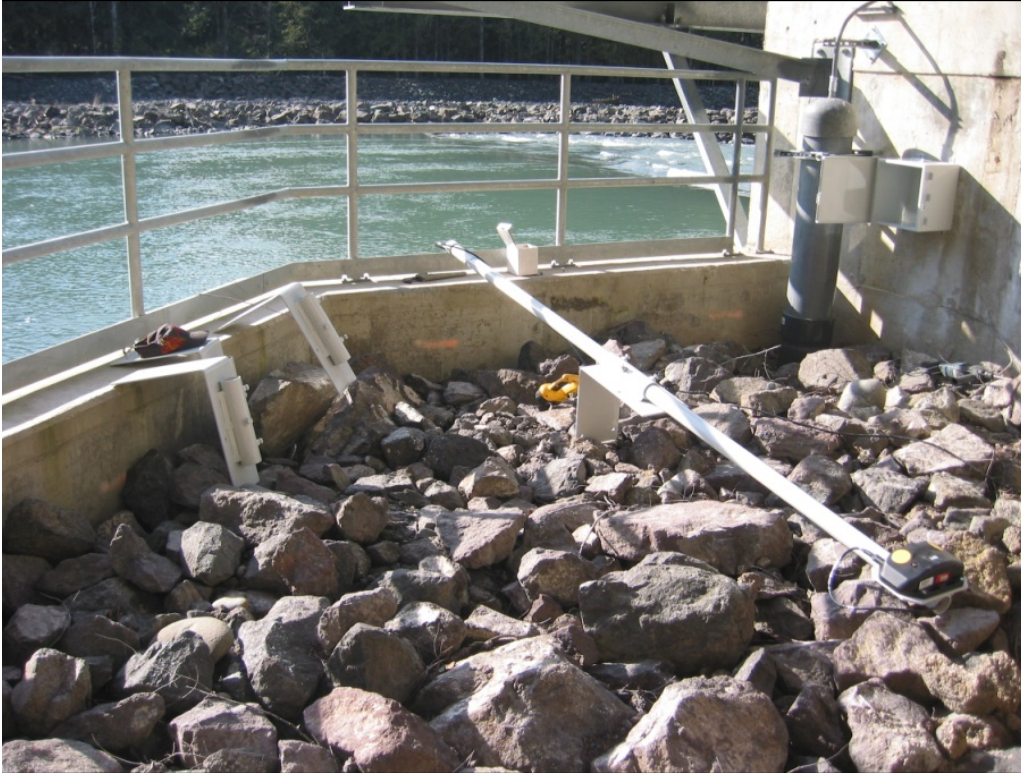
Figure 13. USGS gage (12046260) at the surface water intake provided real-time turbidity and river stage for the Elwha Water Treatment Plant at approximately river mile 3.5.
