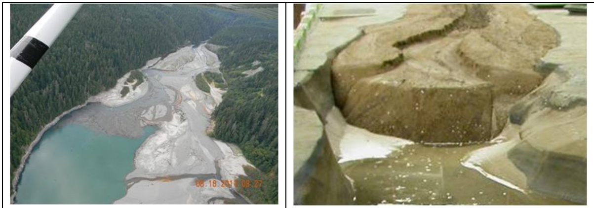
Figure 4. Photographs of the delta sweep showing actual sediment erosion and redeposition at Lake Mills as of August 2011 (16 ft of spillway drawdown prior to dam removal) and a laboratory model of Lake Mills (Bromley, 2007).
