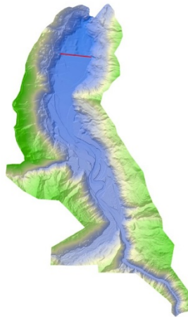
Figure 28. Lake Mills simulation after 109 ft of drawdown on 2012-Oct-07.
