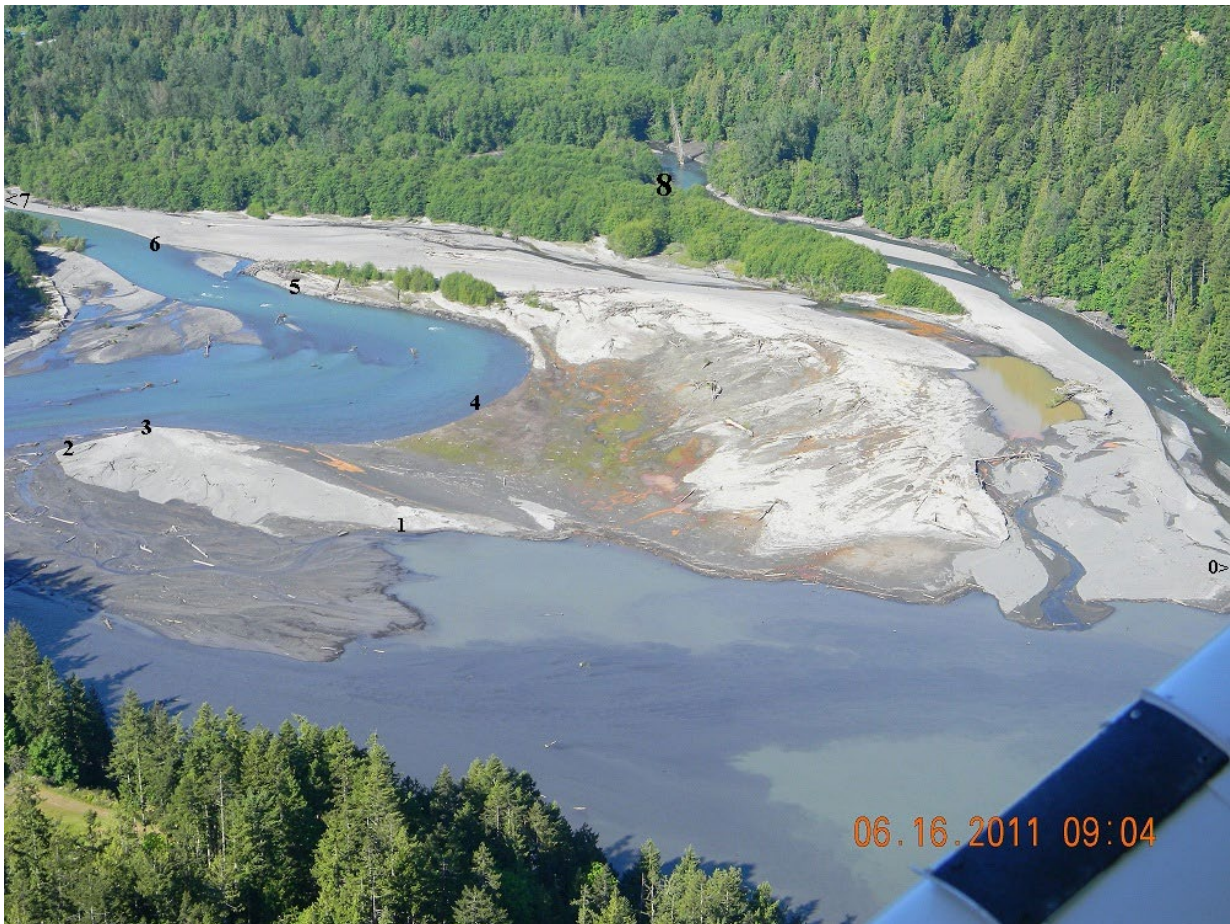
Figure 11. Oblique aerial photograph of points along the eroding Lake Aldwell delta channel during the initial reservoir drawdown, prior to the start of dam removal. Photograph courtesy of Richard Bauman from the Elwha Project Office.
