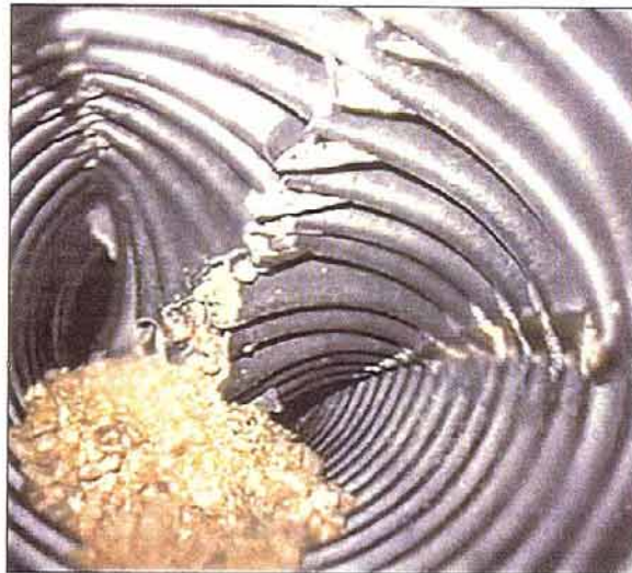
Figure D-6. —HDPE pipe experiencing failure at the crown. Materials surrounding the pipe have entered through the failure.
