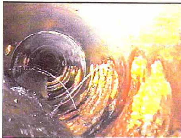
Figure D-15. —Mineral incrustation has resulted in plugging of a number of the pipe perforations.
