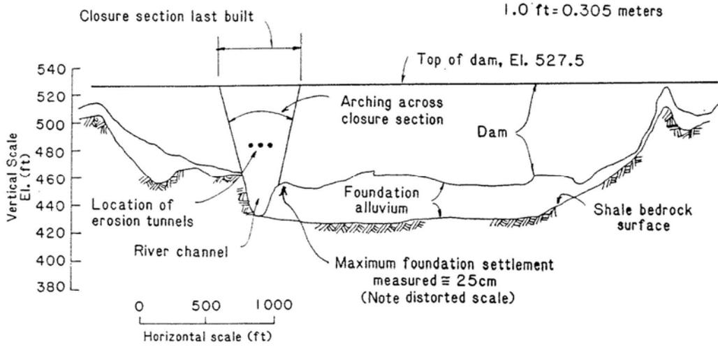
Figure 4. – Examples of Cracking Along a River Channel (Sherard).
