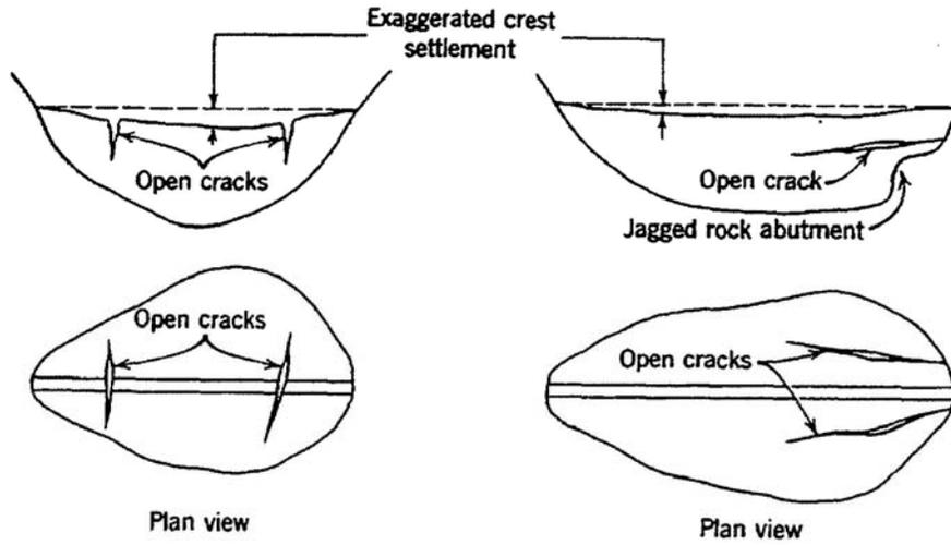
Figure 1A. – Typical transverse differential settlement cracks
