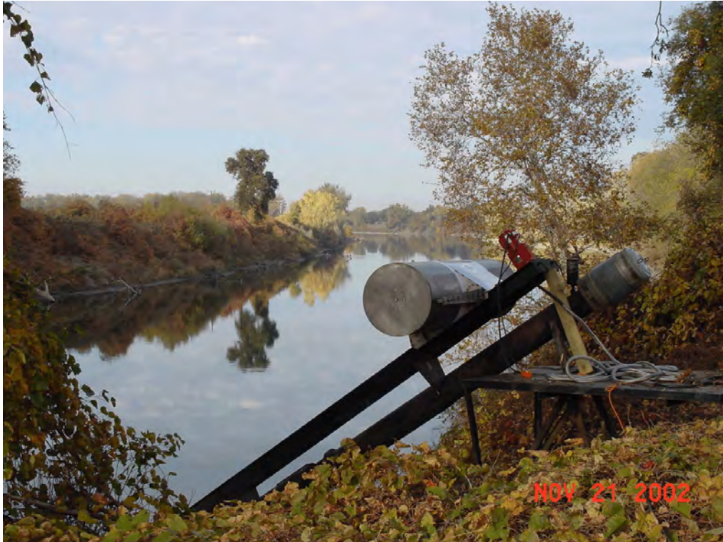
Figure 17.—Track mounted, retrievable rotating cylindrical screen with fixed brush cleaner (intake screens incorporated).
