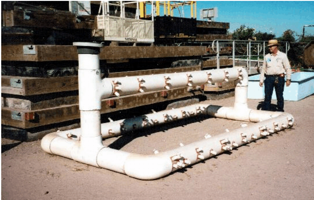
Figure 60.—Air burst device placed in the bay immediately downstream from the Wilkins Slough Fish Screen (RD-108).
