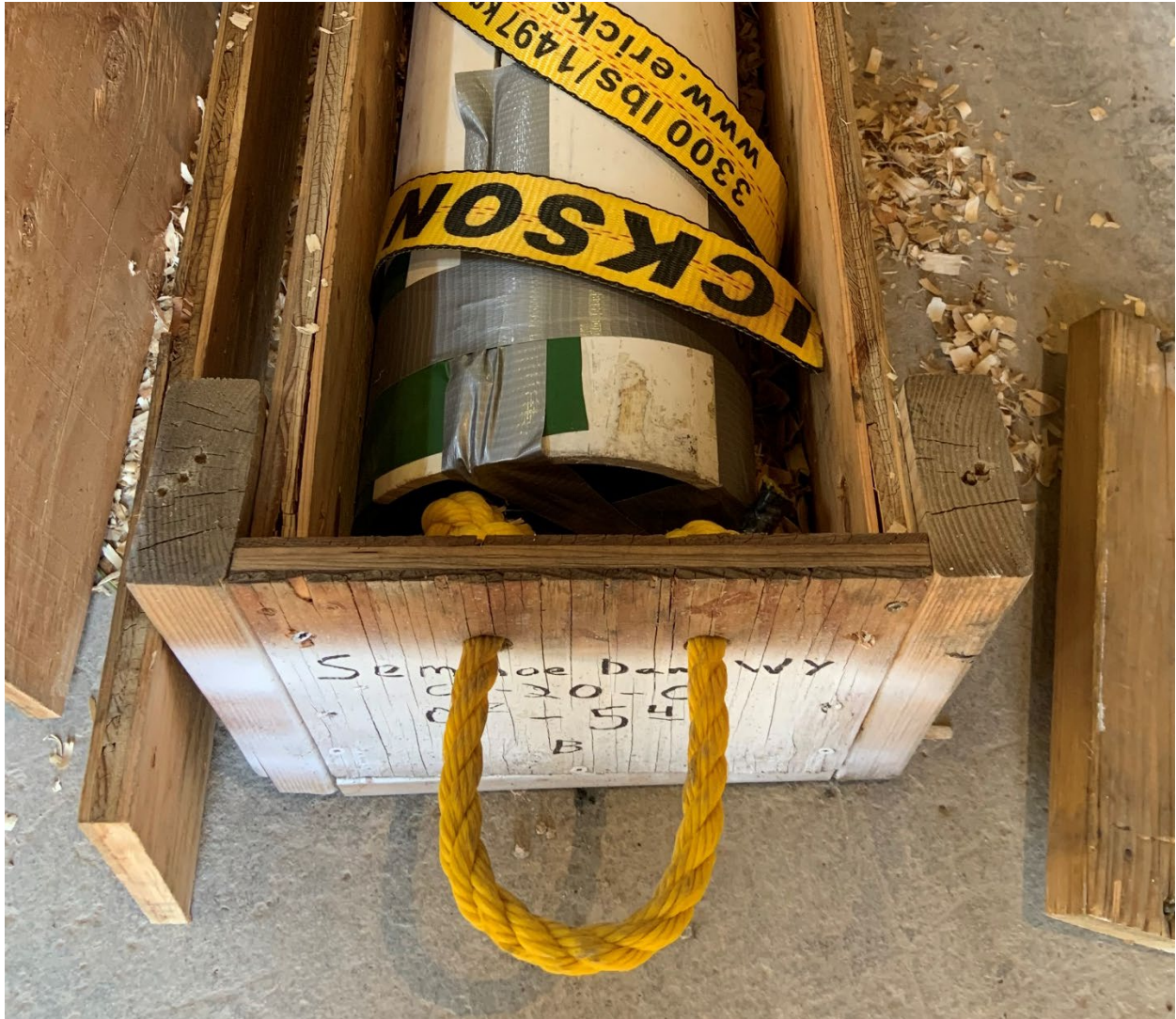
Figure 9. Handles and straps are helpful when moving boxes and sections of core
