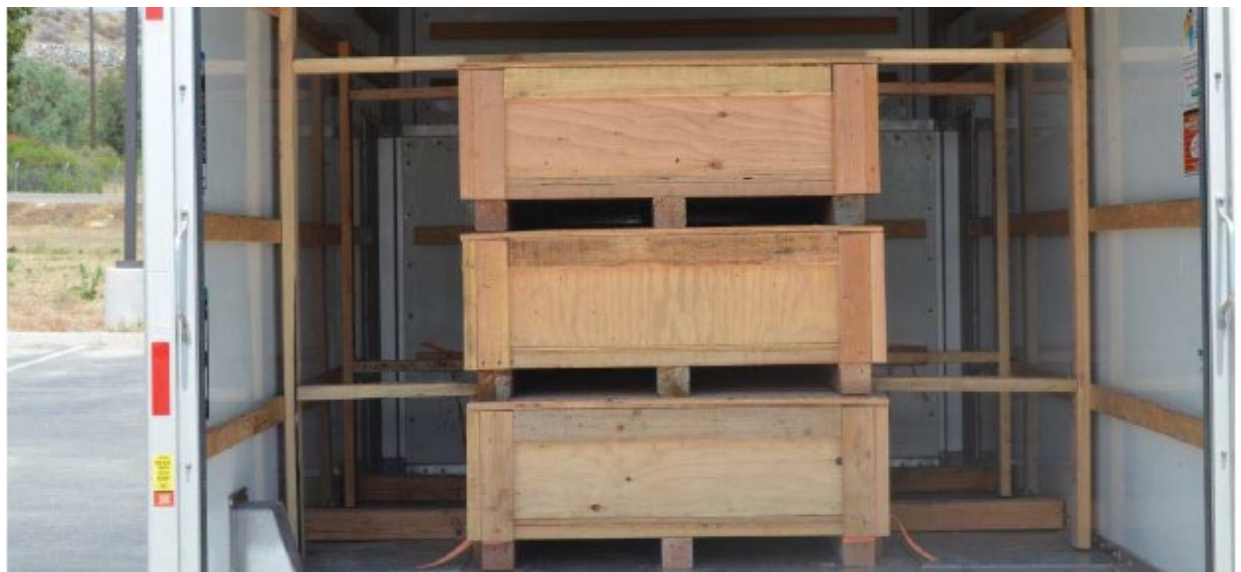
Figure 19. Core boxes secured in enclosed trailer for winter transport (note cross bracing)
