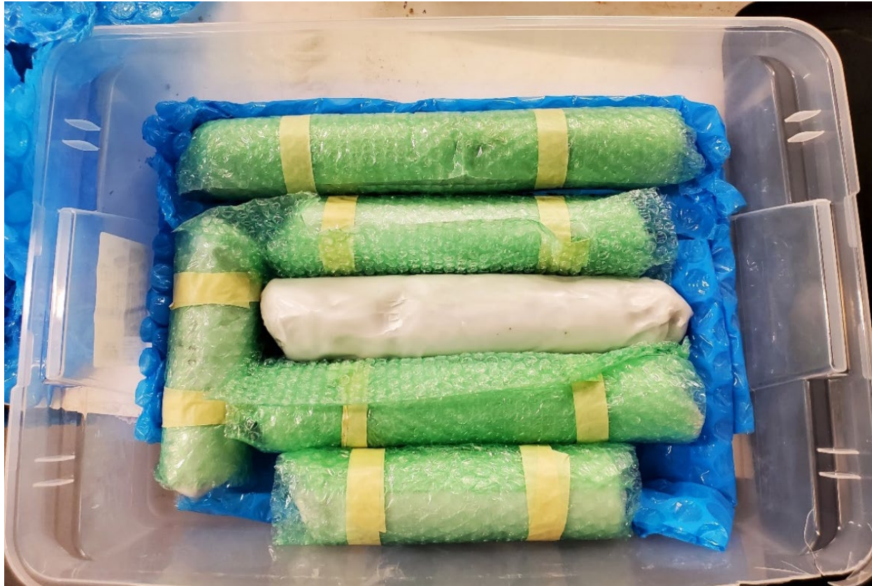
Figure 13. Waxed samples shipped to the laboratory in a plastic box
