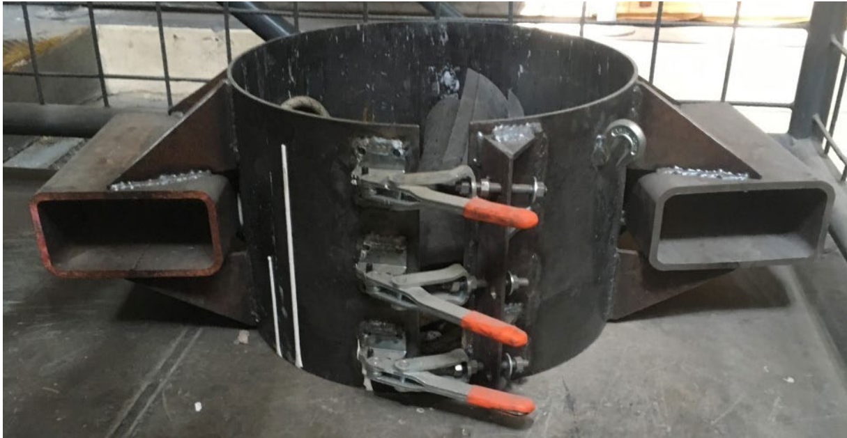
Figure 25. Core clamp with forklift attachment, used for transporting large diameter samples
