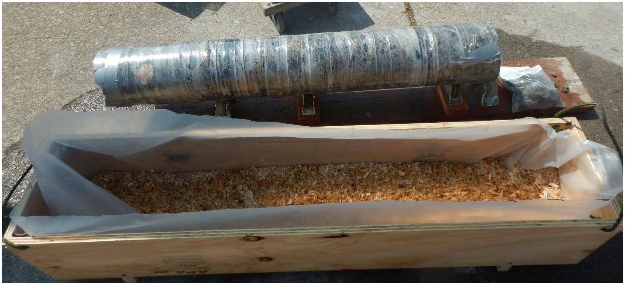
Figure 8. Wrapped with plastic on rolling jig, loaded into box with plastic and dampened wood shavings
