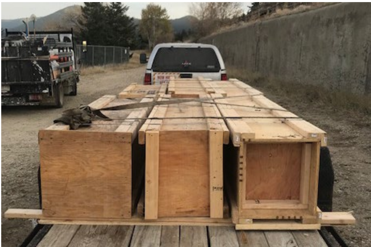
Figure 17. Straps properly securing boxes during transportation
