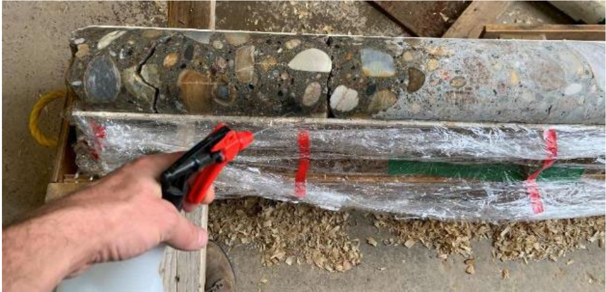
Figure 4. Reapplying moisture and preparing core for shipping
