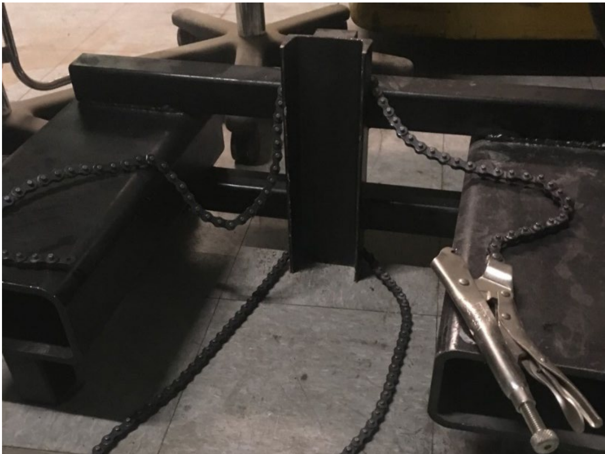
Figure 26. Core grabber with two chains and chain vise grip clamps for forklift
