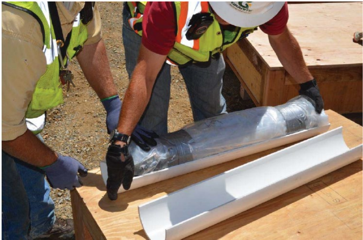
Figure 6. Plastic half rounds to secure cores in the field
