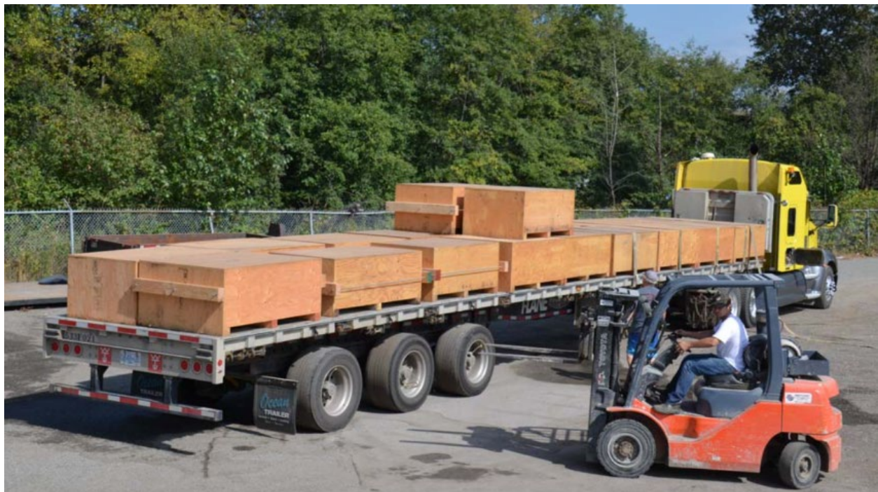
Figure 16. Large diameter concrete core boxes secured to a trailer (note straps being added closest to cab)
