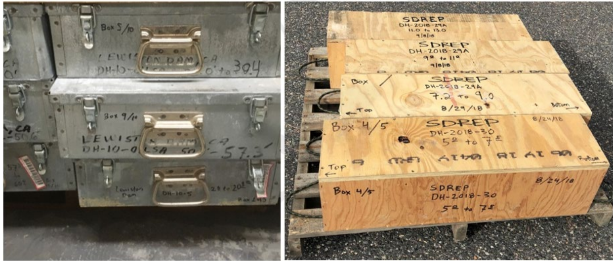
Figure 2. Core boxes labelled with the core hole location and range of depth
