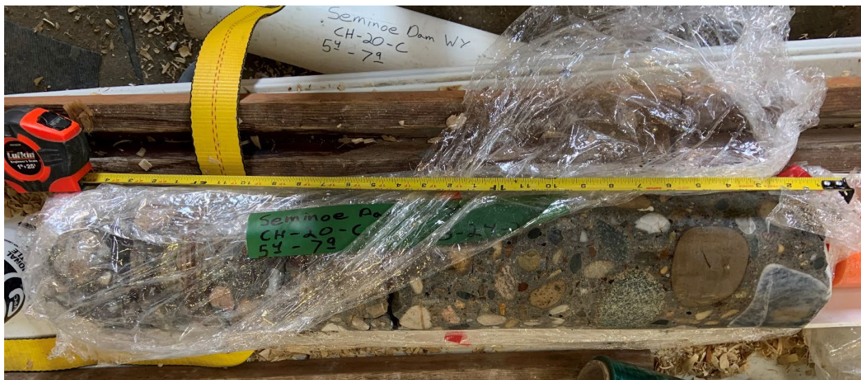
Figure 1. Concrete core with core hole location and depth labeled on plastic wrap
