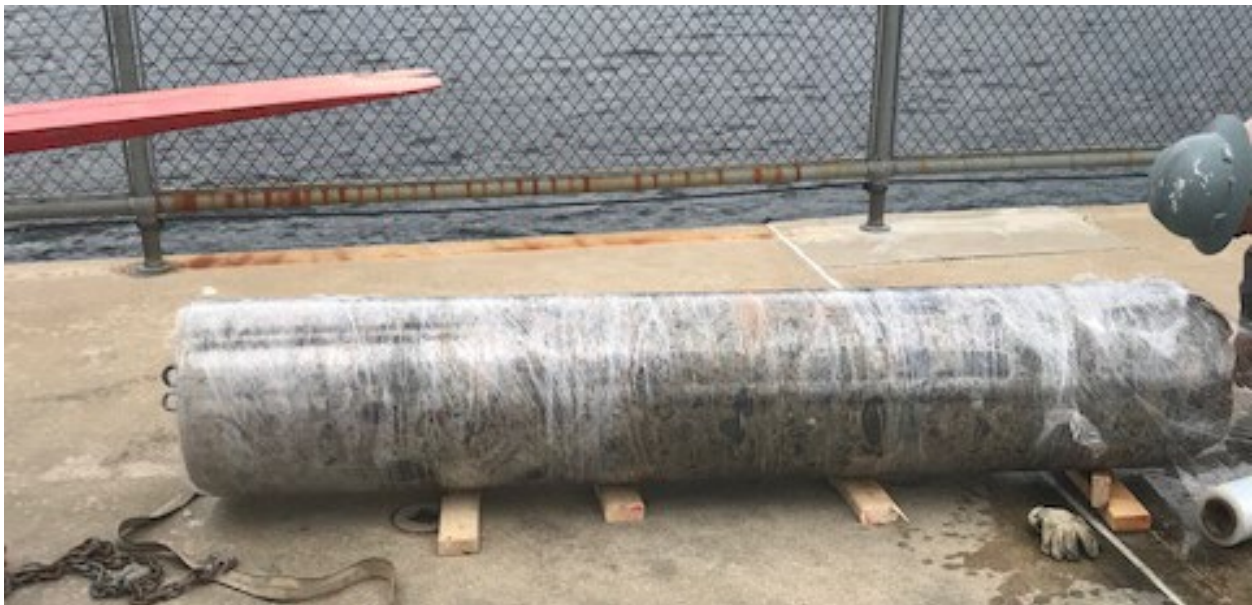
Figure 5. Core sample wrapped with plastic and placed on supports prior to shipping
