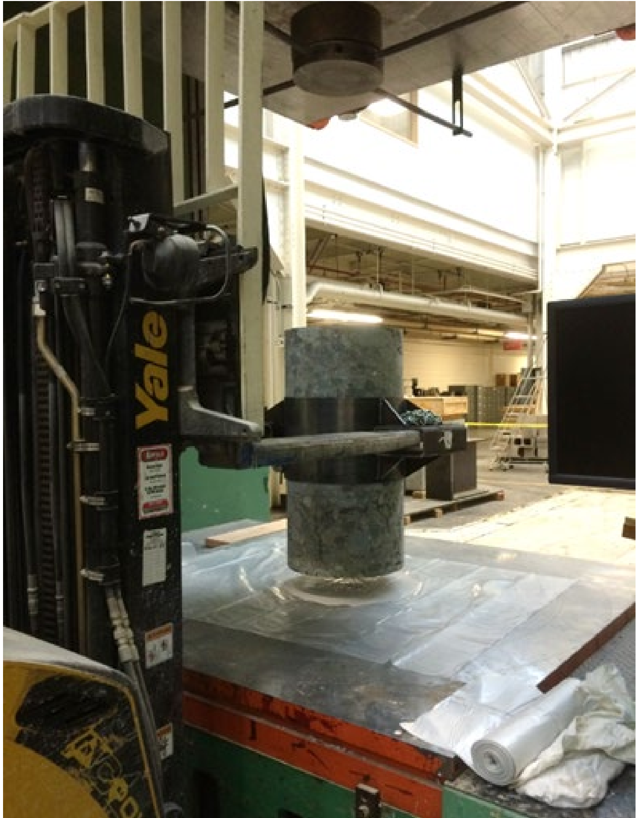
Figure 24. Placing an 18- inch diameter core under the 5-million-pound press for compression testing
