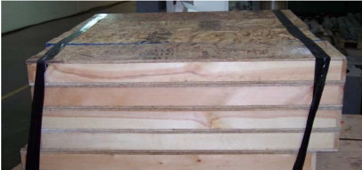
Figure 18. Duct tape used to "strap" sample containers enables shifting
