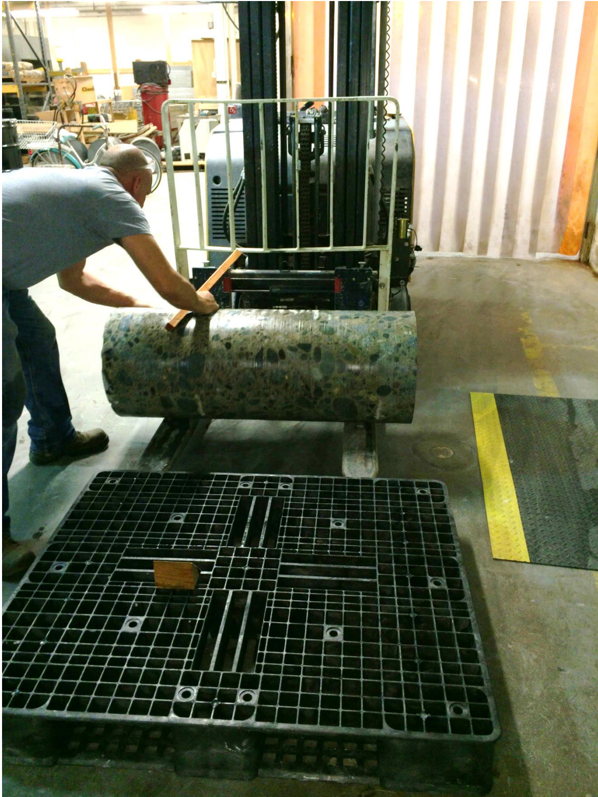
Figure 27. Rolling core horizontally to a pallet with forklift and wedges
