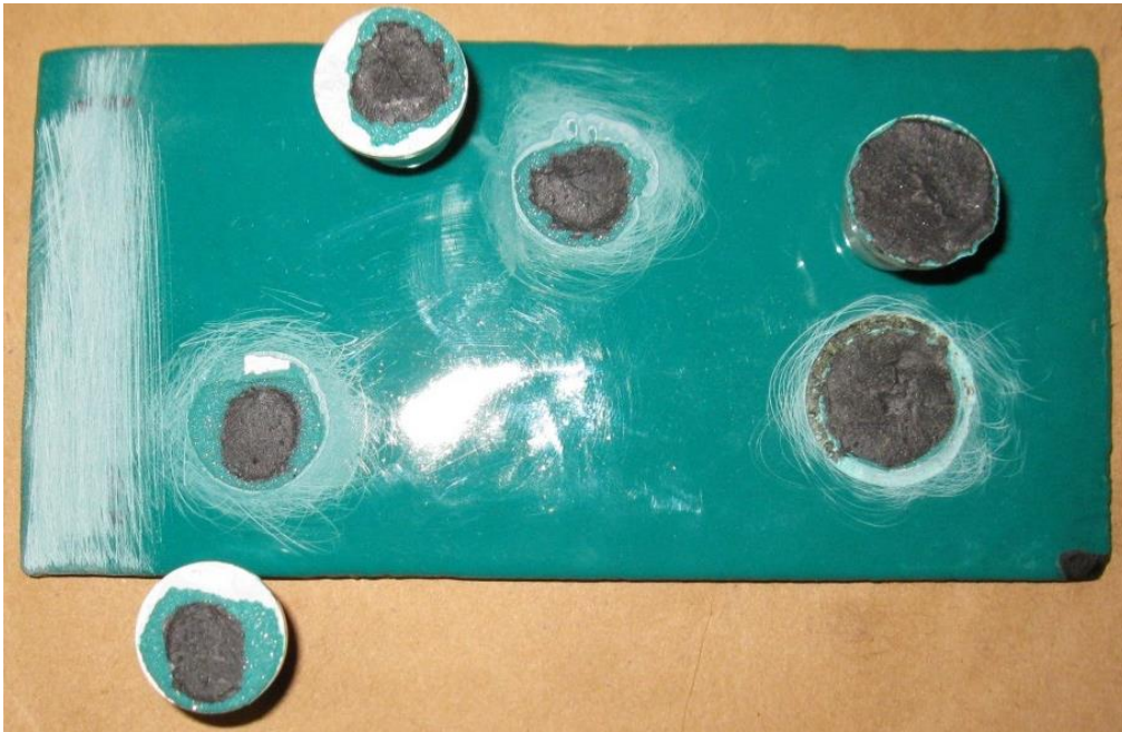
Figure 1-4. Adhesion between coal tar enamel and Powercrete F-1, depicting failure within the coal tar enamel. Black coating is coal tar enamel, turquoise coating is Powercrete F-1 (100% solids epoxy), and the white is the aluminum dolly.
