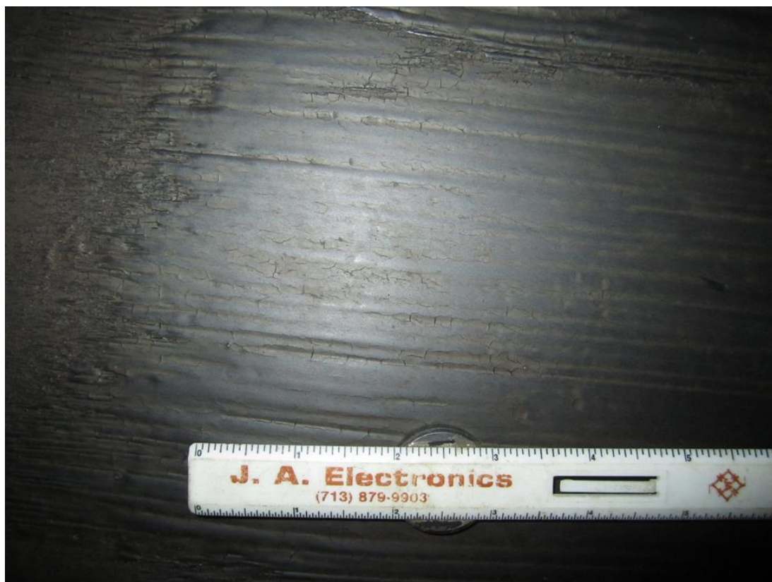
Figure 4. Early stages of cracking that are visible only on the coating’s surface and do not penetrate down to the substrate.
