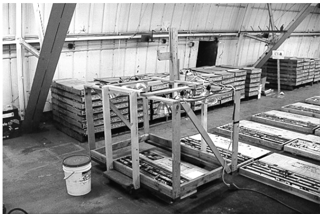
Figure 23-2.—Core storage area with boxes neatly arranged and separated by spacers for ventilation. Note core photography frame in center of photograph.
