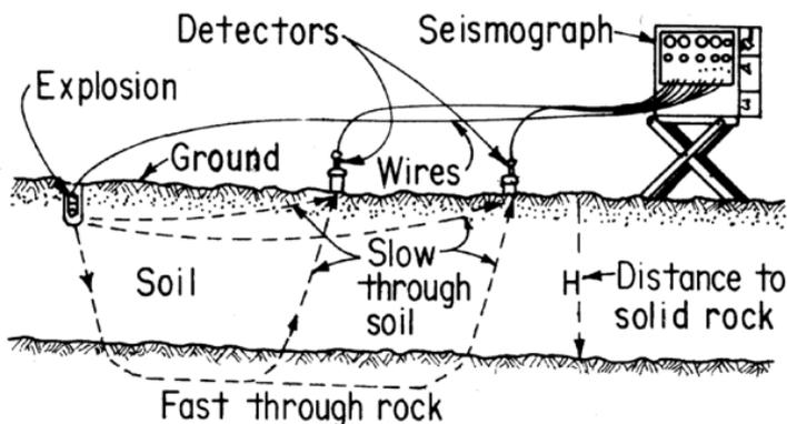
**Figure 13-1.—Simplified diagram of a seismic refraction test.**
