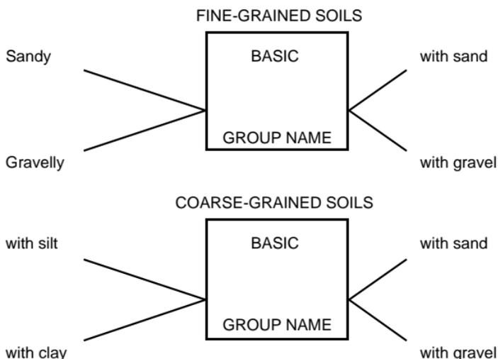
Figure 3-1.—Modifiers to basic soil group names (for visual classification).
