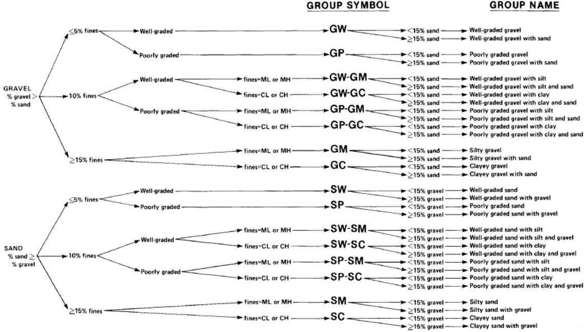
Figure 3-4.—Flow chart for coarse-grained soils, visual method.
